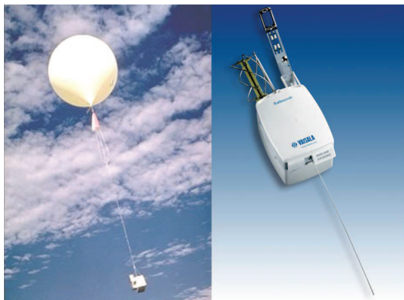
Figure 2-9: Balloon with an attached radiosonde together with a close-up of the Vaisala Radiosonde RS92. (Vaisala, 2006)
