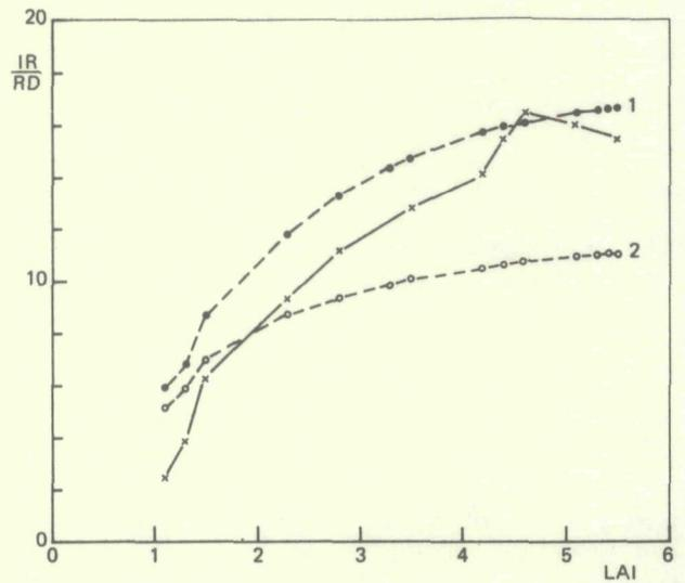
Fig. 2 Comparison between the IR/RD hot-spot reflectance ratio as measured for the vegetative phase of winter wheat (Durin) with model simulations for dark green(1) and light green(2) leaves
