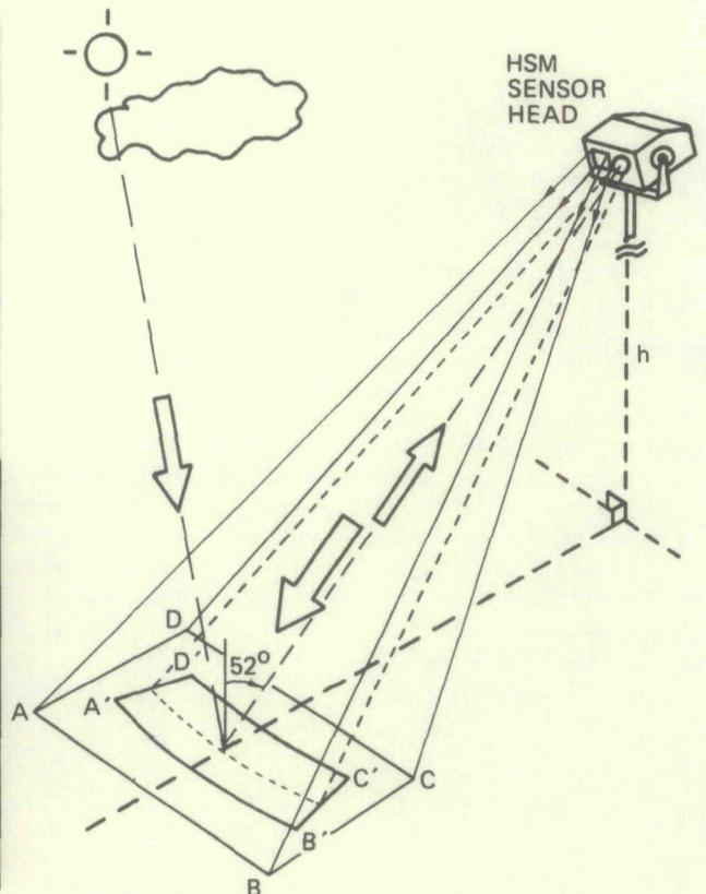
Fig. 4 HSM-measurement configuration. The area ABCD is illuminated by the radiant source. Hot-spot reflectance is measured within the sensor field of view with footprint A'B'C'D'
