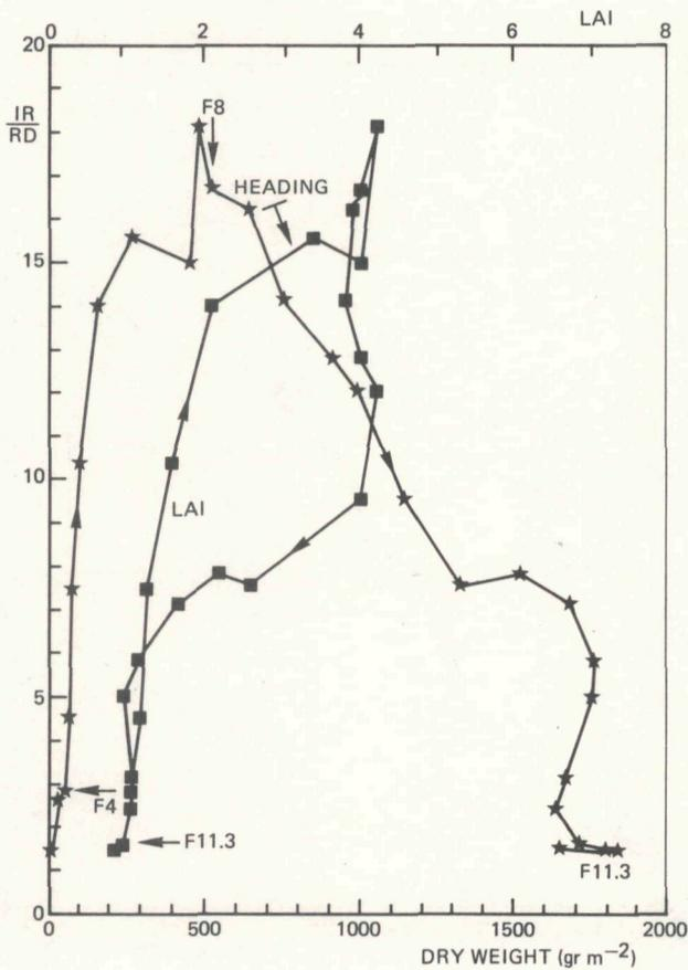
Fig. 7 HSM IR/RD reflectance ratio of winter wheat (Adamant) as a function of the measured LAI and total dry weight
