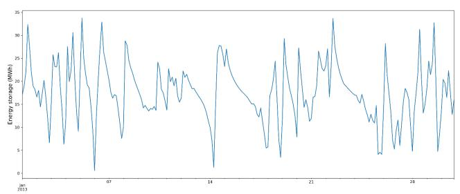
Figure 27: modeled state of charge of battery energy storage in January 2013 in the baseline scenario.
