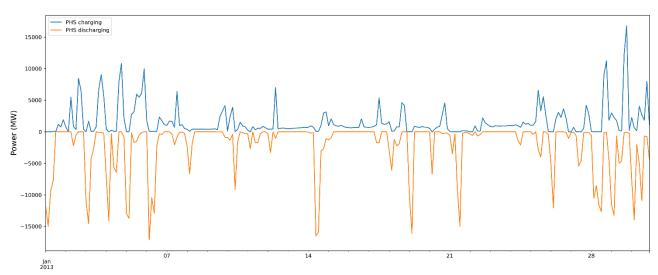
Figure 31: electricity generation and consumption of pumped-storage hydroelectricity in January 2013 in the baseline scenario.
