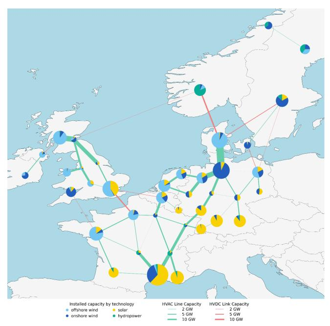
Figure 7: power plant capacity per node and transmission system expansion in the baseline scenario.
