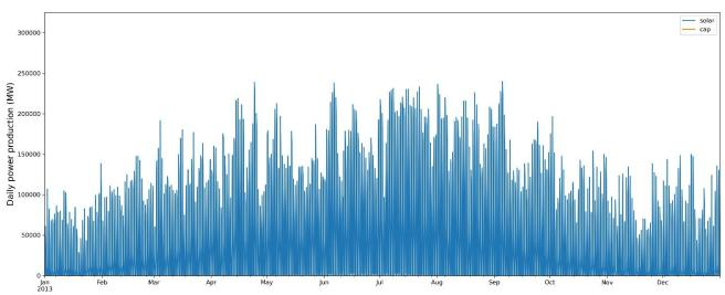
Figure 18: modeled aggregated solar PV electricity generation in the North Sea countries in the baseline scenario. The horizontal orange line denotes the solar PV capacity.
