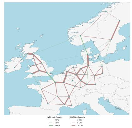
Figure 6: PyPSA-Eur model of the electricity system of the North Sea countries including all existing high-voltage alternating current (HVAC) and high-voltage direct current (HVDC) lines.
