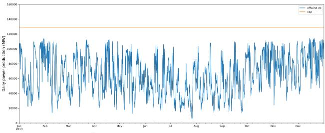
Figure 21: modeled aggregated offshore wind electricity generation connected by DC lines in the North Sea countries in the baseline scenario. The horizontal orange line denotes the offshore wind capacity installed via an alternating current connection line.
