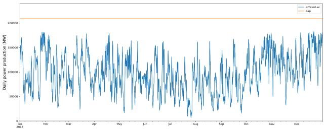
Figure 20: modeled aggregated offshore wind electricity generation connected by AC lines in the North Sea countries in the baseline scenario. The horizontal orange line denotes the offshore wind capacity installed via an alternating current connection line.
