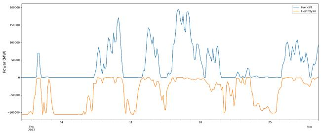
Figure 29: electricity generation of fuel cells by burning hydrogen and electricity consumed to produce hydrogen by electrolyzers in the baseline scenario in February 2013.
