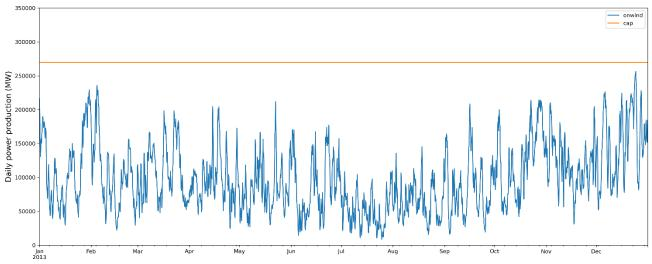
Figure 19: modeled aggregated onshore wind electricity generation in the North Sea countries in the baseline scenario. The horizontal orange line denotes the onshore wind power capacity.
