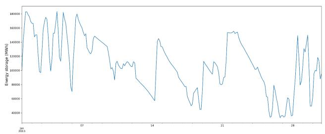
Figure 28: modeled state of charge of the pumped hydro energy storage in January 2013 in the baseline scenario.
