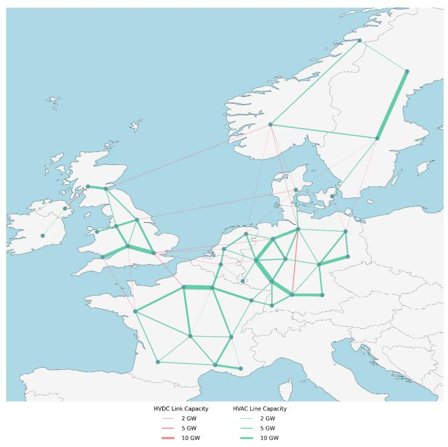
Figure 16: lay-out of the transmission network of scenario 2. In this scenario, no network expansion is allowed.
