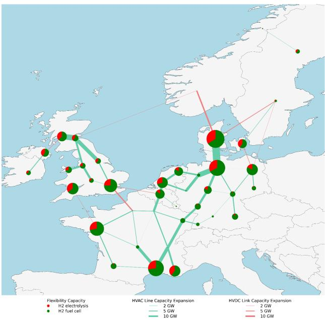
Figure 10: hydrogen electrolysis capacity, hydrogen fuel cell capacity, and the transmission network expansion of the baseline scenario.
