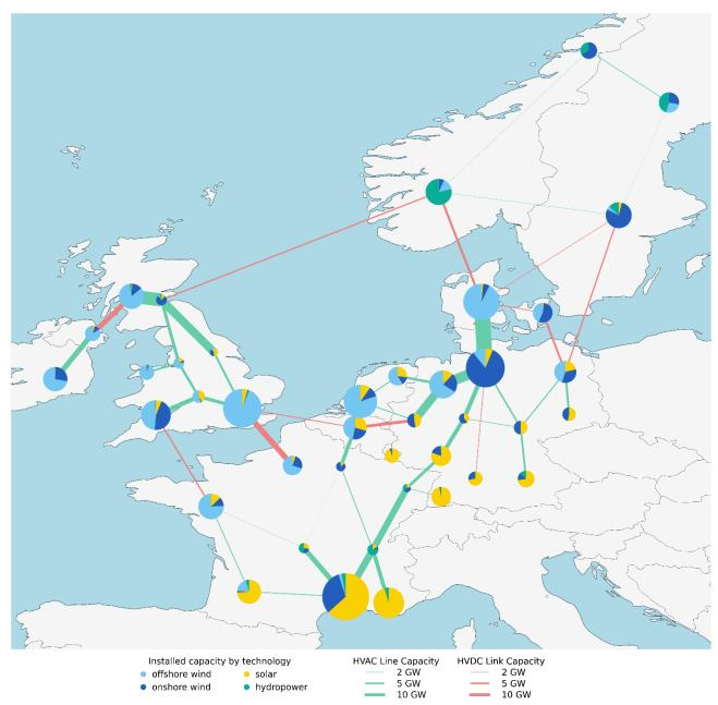
Figure 17: lay-out of the transmission network of scenario 13. In scenario 13, tank storage is used to store hydrogen instead of salt caverns.
