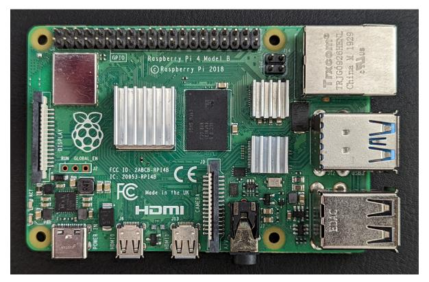
Figure 4.1: The Raspberry Pi 4 used with heatsink placement.
