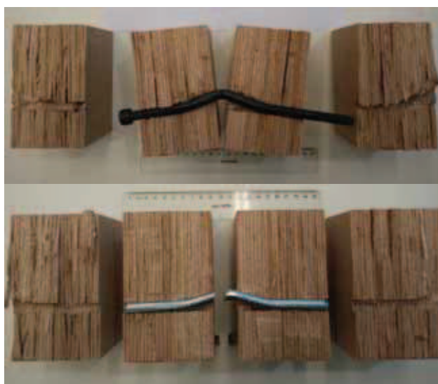
Figure 13: Beech LVL joints: slotted in steel plate with single dowel. Upper: HSS grade 12.9, Lower: ordinary steel grade S235. (Steel plate not shown).
