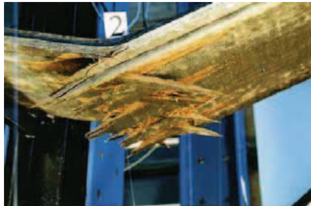
Figure 1: Cross grain in an azobé board loaded in flatwise bending.
