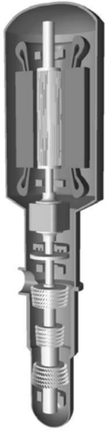
Figure 2.2 Schematic cross-section of a turbo-generator for a nuclear power plant, the first pebble-bed high temperature gas-cooled test reactor with the gas turbine in the direct cycle (HTR-10GT, under construction, Chinese government key project): 6 MW, 15000 rpm, vertical rotor axis, 4 radial bearings, 2 axial bearings, length of turbine 3.5 m, mass of turbine 1000 kg. (photo courtesy Institute of Nuclear and Novel Energy Technology INET, Tsinghua University, Beijing, [11]).
