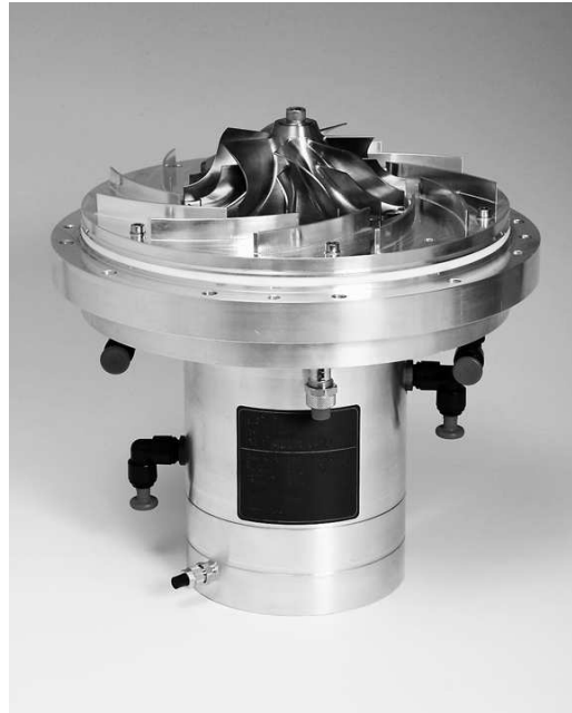
Figure 2.3 Turbo-blower: cooling gas compressor ( \text{CO}_2 ) for a power laser, cutting a metal sheets up to 25mm. The laser needs uncontaminated gas. The speed is 54000 rpm, the rotor mass 3.6 kg, the motor power 12 KW, the radial bearing 48 mm in diameter, the bearing force 230 N (photo courtesy TRUMPF/MECOS) [10].
