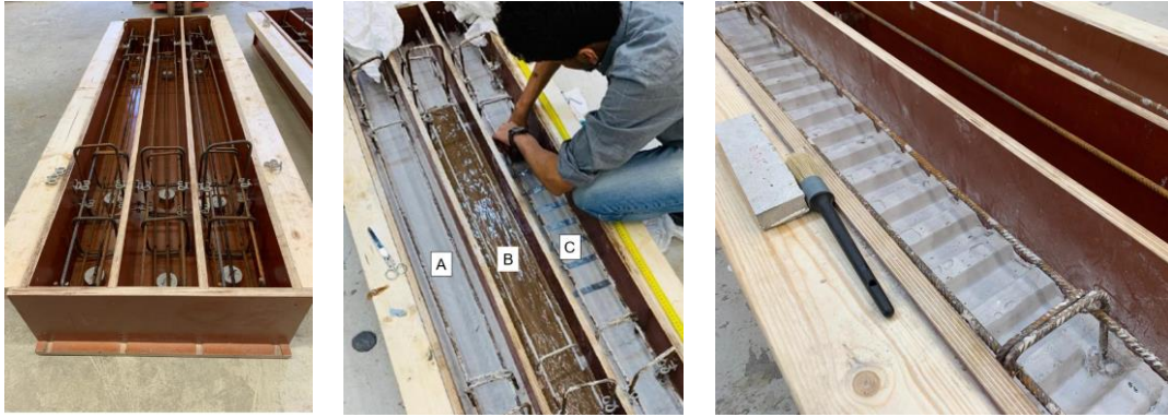
Figure 3. Plywood moulds with reinforcement cage and SHCC spacers (left). Smooth (A), completely delaminated (B) and partially delaminated (C) surfaces (middle). Profiled surface (right).
