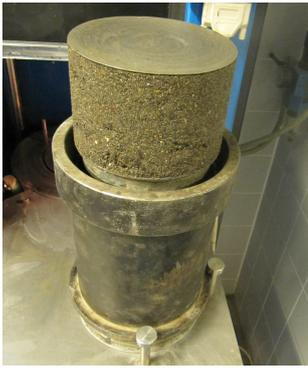
**Figure 3.10:** Extraction from SGC mould
