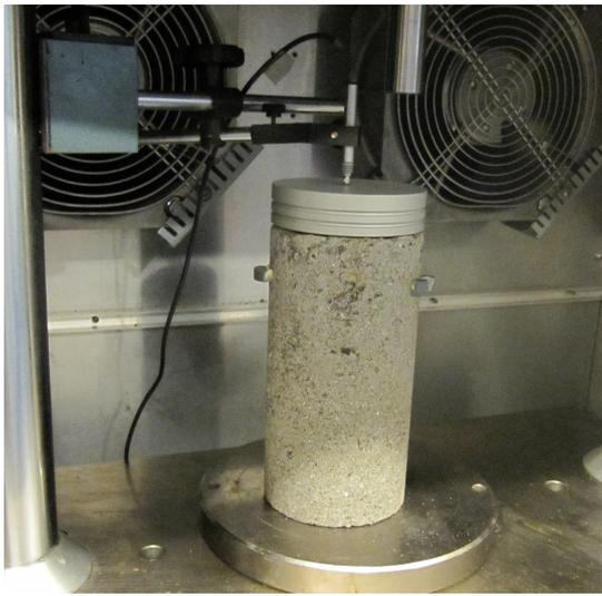
Figure 3.29: Thermal deformation test set-up
