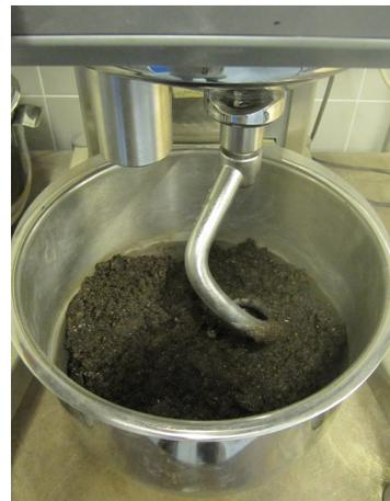
**Figure 3.5:** The mix blended with water and cement
