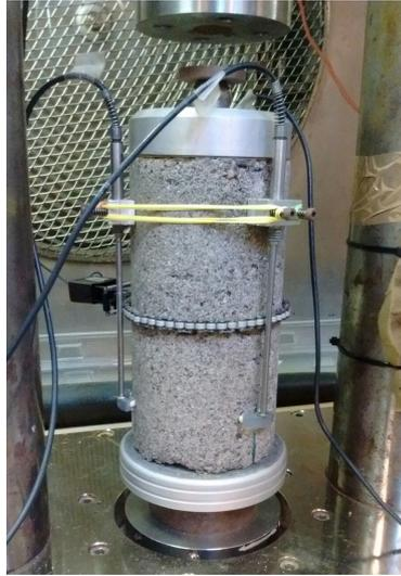
Figure 3.33: Poisson's test set-up
