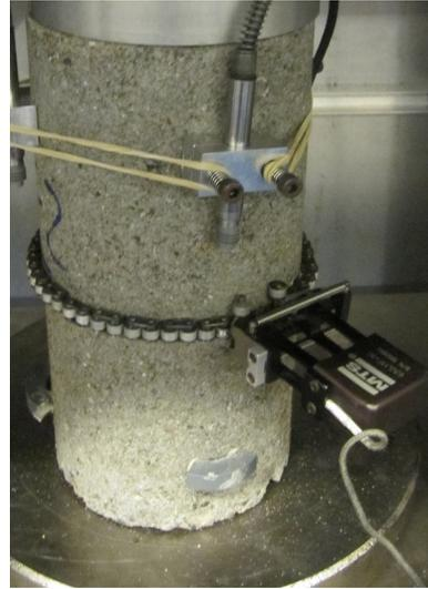
Figure 3.34: Detail of the chain device
