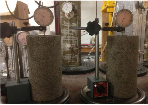
Figure 3.22: Shrinkage test set-up
