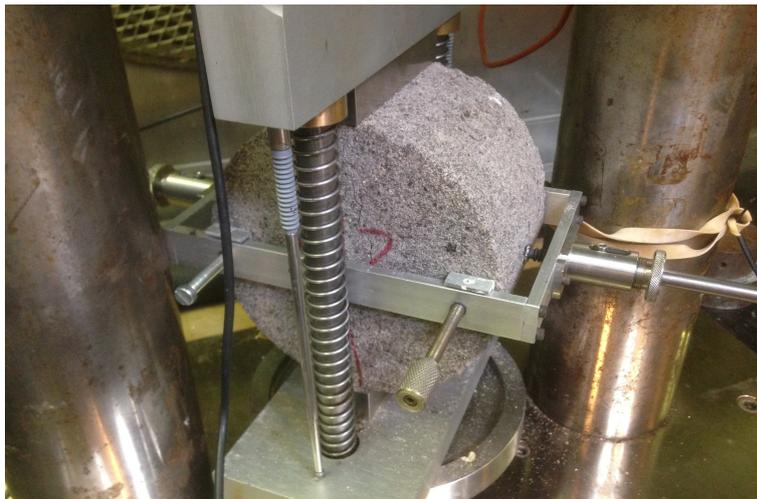
Figure 3.40: ITT test set-up
