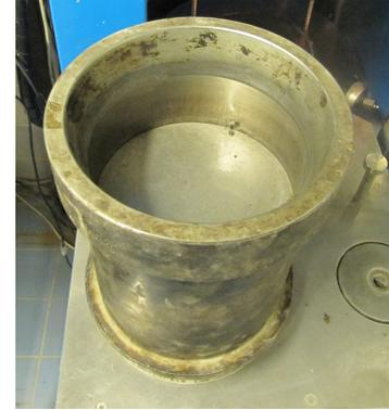
**Figure 3.8:** SGC mould preparation - step 3/3
