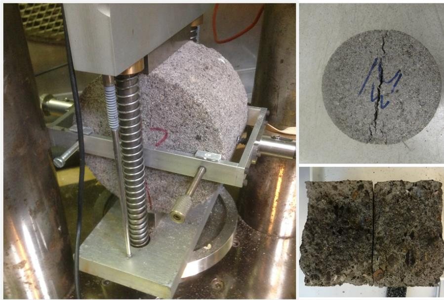
**Figure 3.16:** ITT test set-up and photos of a cracked sample
