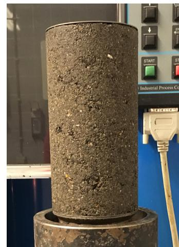
**Figure 3.14:** The sample is extracted from the mould
