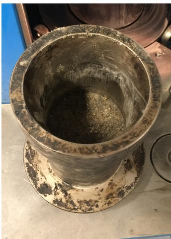
**Figure 3.12:** Compaction of the first third of the sample
