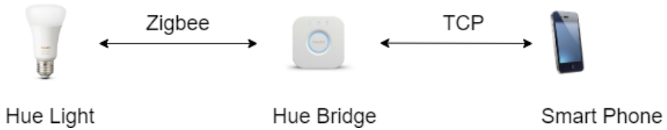
Figure 8.1: Hue bridge uses Zigbee to communicate with lights whereas it uses TCP to communicate with smart phone controlling it.
