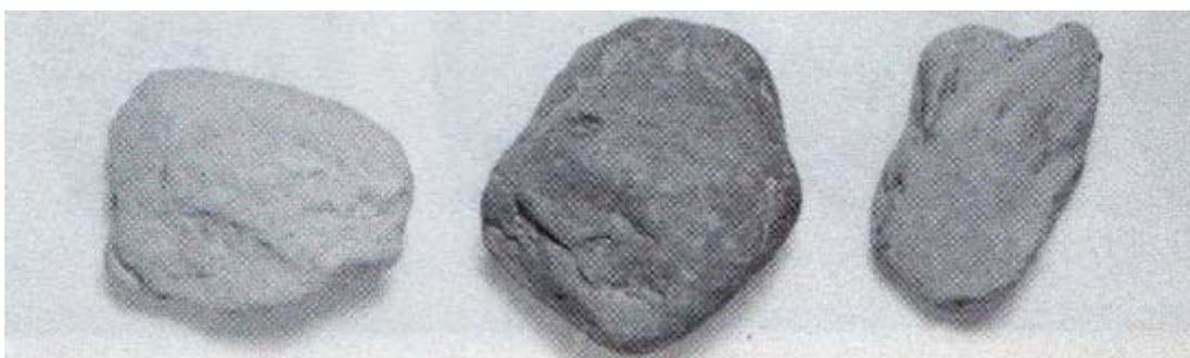
**Figure 2.12: Riprap after 134 tests, 2x painted**
