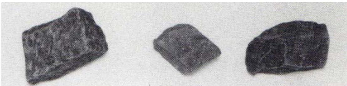
**Figure 2.16: Basalt after 10 tests, not painted**
