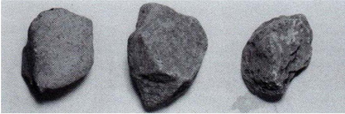
**Figure 2.13: Uniform stone after 106 tests, 1x painted**
