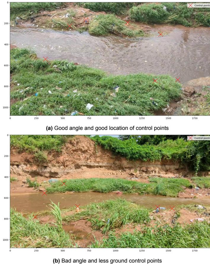
**Figure 6.1:** Tamale camera views with different angles and number of control points. The red crosses show the control points.
