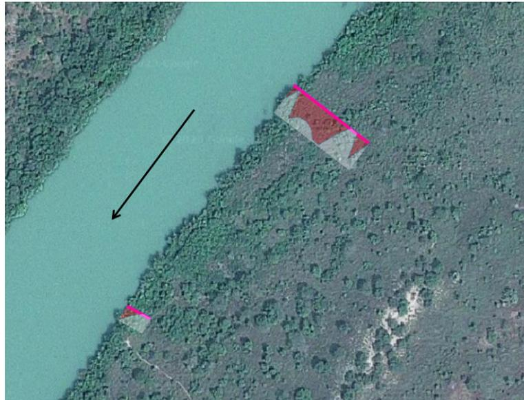
**Figure 7.6:** Two velocity profiles that were obtained in the floodplain using a current meter. The height of the red part of the graph gives the measured velocity at the location along the bright-pink line in the direction of the river (black arrow). The white portion gives the highest velocity measured along the transect. This is 0.38 and 0.15  $m/s$  for the upstream and downstream transect respectively.
