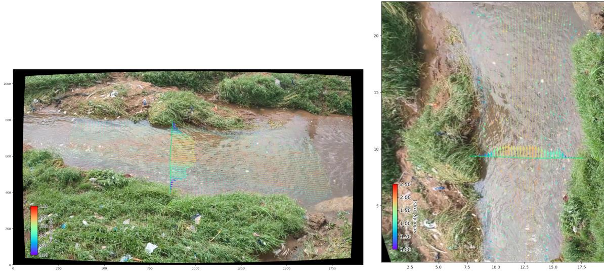
Figure 6.7: Tamale velocimetry without lens position higher camera view (left) and top view projection (right)
