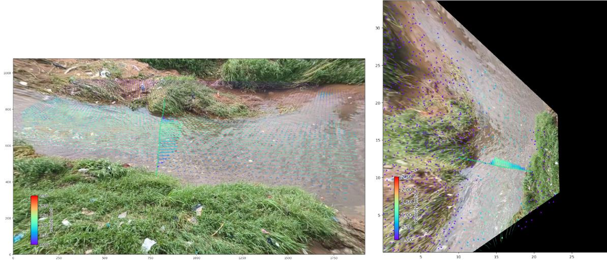
Figure 6.8: Tamale velocimetry with lens position and higher camera view (left) and top view projection (right)
