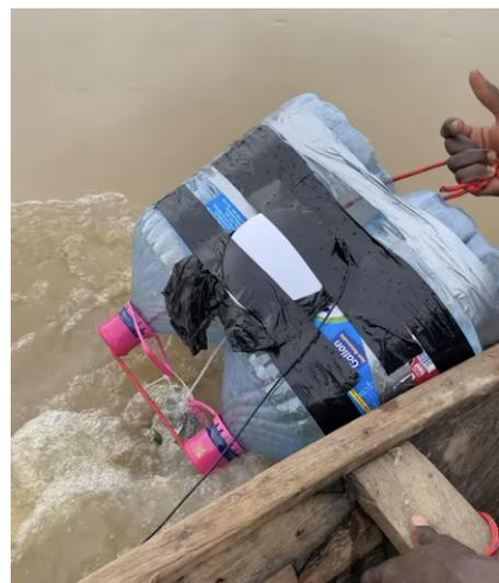
(b) Set-up of Deeper Sonar Chirp+ device on floaters.
