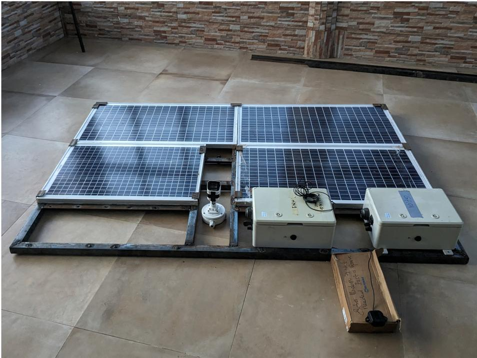
**Figure A.2:** Platform for sensor setup on the pole in Chache.
