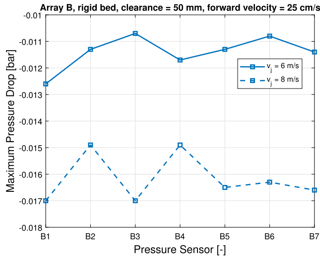
Fig. 23. Effect of jet velocity (left) and forward velocity (right) on the maximum pressure drop under the collector; v_j is jet velocity and v_f is the forward velocity of the collector.
