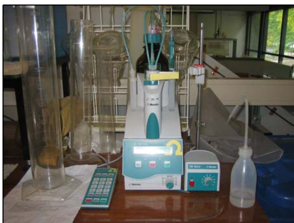
Figure 4.4. (a) Apparatus for m- number analysis (b) Apparatus for calcium analysis
