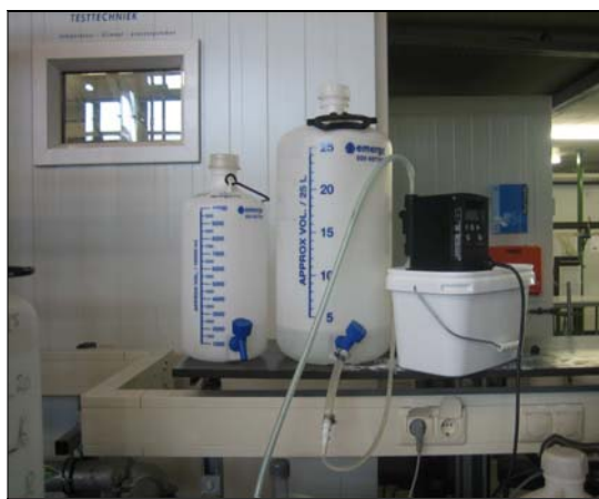
Figure 4.4 Dosage tanks with \text{Na}_2\text{CO}_3 solution (left) and \text{HCl} solution (right)
