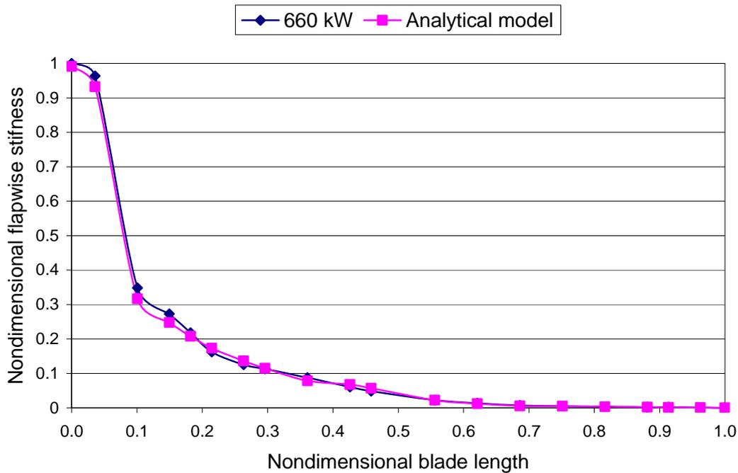
Figure 2: Comparison of flapwise stiffness of the analytical model with the 660 kW wind turbine blade
