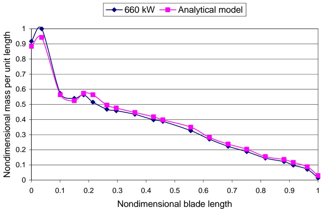
Figure 4: Comparison of mass per unit length of the analytical model with the 660 kW wind turbine blade
