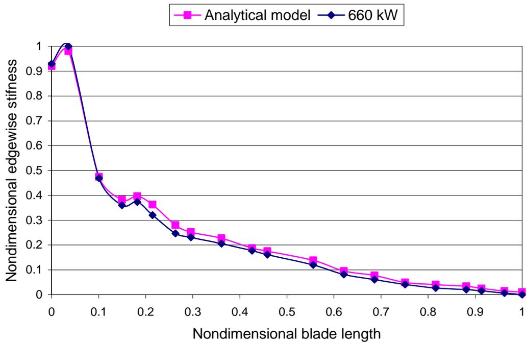
Figure 3: Comparison of edgewise stiffness of the analytical model with the 660 kW wind turbine blade
