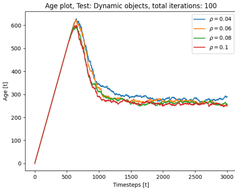
Figure 4-5: Incremental policy with different evaporation factors
