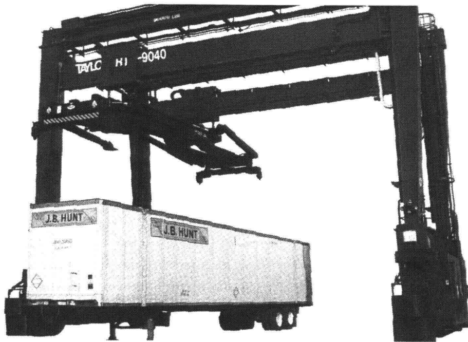
Figure 7-9: Rubber Tyred Gantry (RTG)
