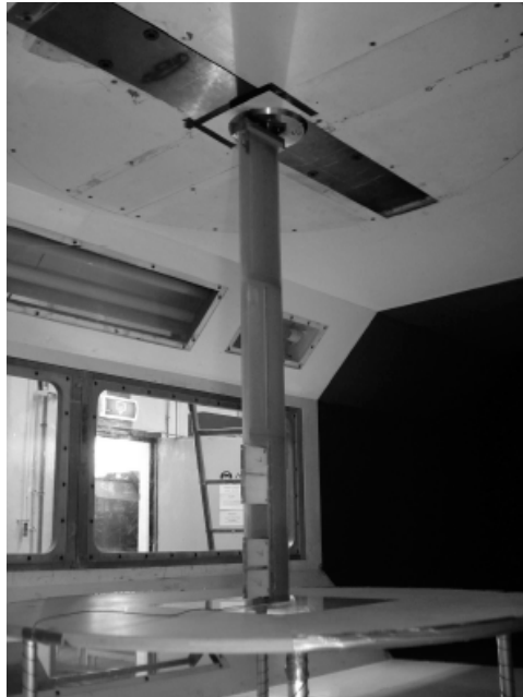
Fig 1: The adaptive blade at the LSLT wind tunnel test section
