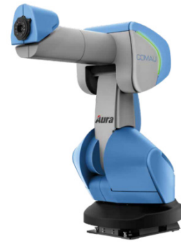
Figure 67: AURA-170-2.8 (170 kg), with industrial and cobot operation mode. Adapted from: Comau (n.d.).
