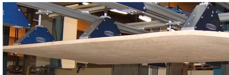
Figure 42: An three by one array of the ingressive gripper type carrying a sheet of fibrous material. Adapted from: Schmalz (2019).
