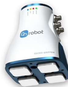
Figure 46: The gripper that is able to mimic the sticking capabilities of a gecko. Reprinted from: On Robot (2019).
