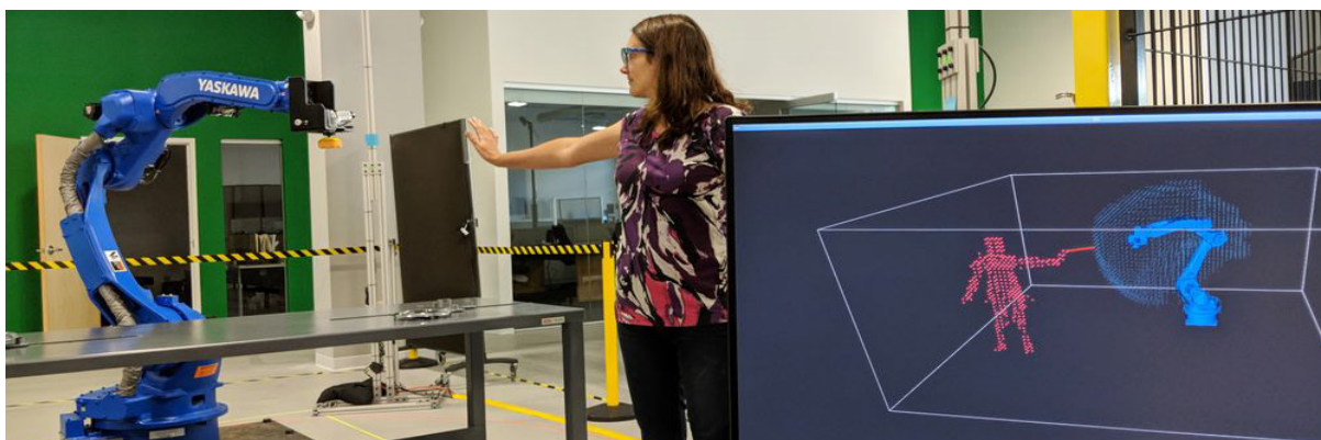
Figure 35: Vision system that uses lidar sensors to enable a safe work environment for humans around industrial robots. Adapted from: Veo Robotics (2019).
