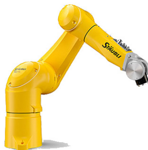
Figure 63: TX2-90L (15 kg), with industrial and cobot operation mode. Adapted from: Stäubli (2019).
