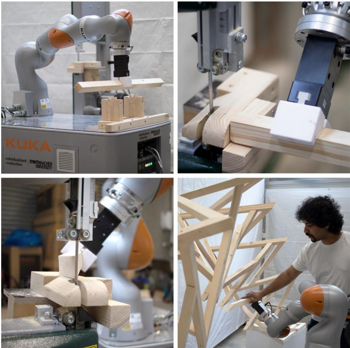
Figure 25: Assembly operation examples pertaining to the main categories of assembly. Upper left: handling; upper right: aligning; lower left: sawing; lower right: positioning. Reprinted from: Stumm et al. (2018).
