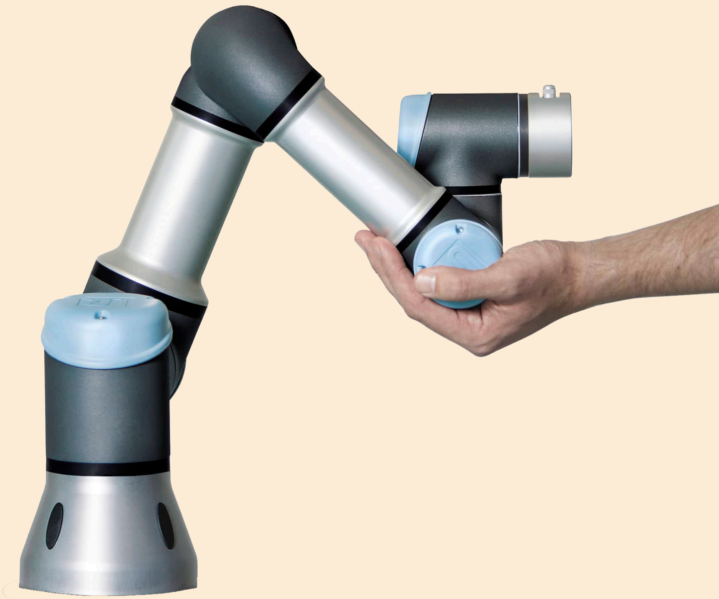
Figure 170: A UR3 collaborative robot can work together with a human. Adapted from: Latmas (n.d.).
