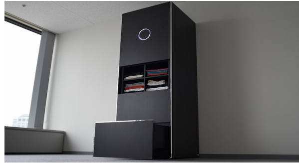
Figure 5: Dried laundry can be dropped in the bottom drawer. Two robot arms will fold the clothes and sort it based on who wears them. Reprinted from: Laundroid (n.d.). Unfortunately, towards the end of the research, the company filed for bankruptcy (Seven Dreamers, 2019).
