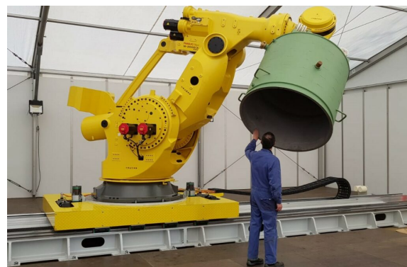
Figure 173: Industrial robot M-2000iA/2300 with a payload capacity of 2.300 kg and a mass of 11.000 kg moves over a rail. Reprinted from: AT-Aandrijftechniek (2019).
