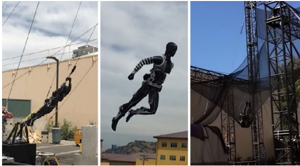
Figure 4: Three steps of the stunt double being launched, flying through the air and landing in a safety net. This prevents the need for stunt doubles to be put through some of these dangerous stunts. Adapted from: Panzarino (2018).
