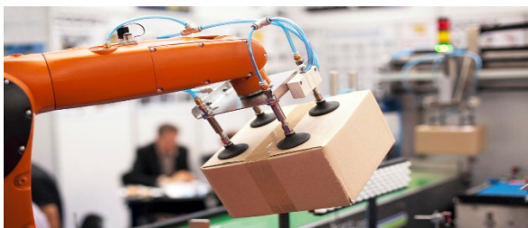
Figure 43: A two by two array of vacuum suction cups lifting a cardboard box. Adapted from: Robotics Online (2019).
