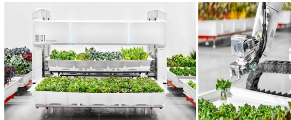
Figure 9: Robot positions a growing container and can plant as well as harvest the crops. Adapted from: Iron Ox (2018).
