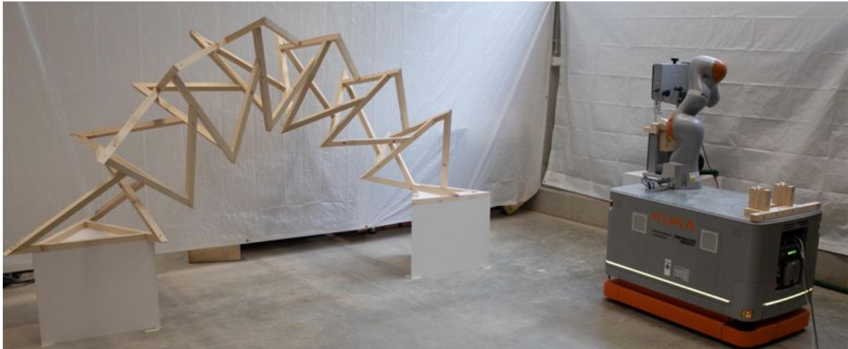
Figure 24: The Twisted Arch is constructed with the help of a KUKA LBR iiwa (LBR refers to “lightweight robot” and iiwa stands for “intelligent industrial work assistant”) which is mounted on a KUKA mobile platform. Reprinted from: Stumm et al. (2018).
