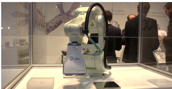
Figure 45: The Gecko gripper moving a small piece of glass at Automatica 2018. Adapted from: On Robot (2019).
