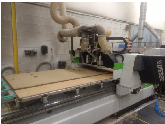
Figure 168: Photo of the CNC milling machine while it is milling the outer layer of geometry version A - Original.
