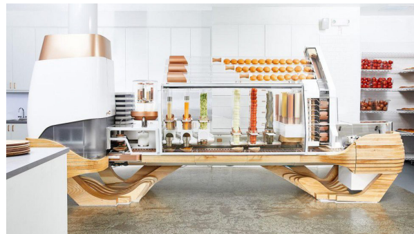
Figure 7: Robot which is able to make 120 hamburgers per hour for $6 each. Reprinted from: Troitino (2018).
