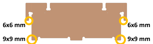
Figure 140: Horizontal beam with the increased chamfers highlighted with orange circles.
