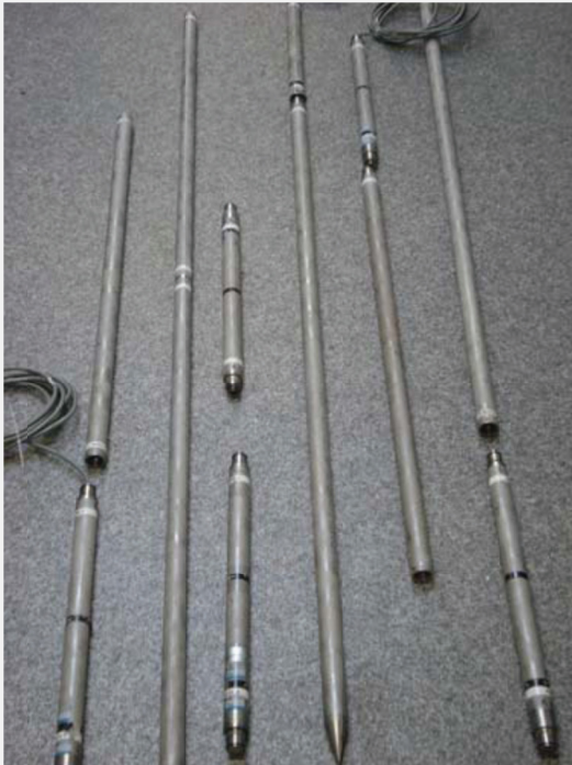
Figure 2-4: SDP sensor modules with rigid connections (Rijkswaterstaat, 2009b)
