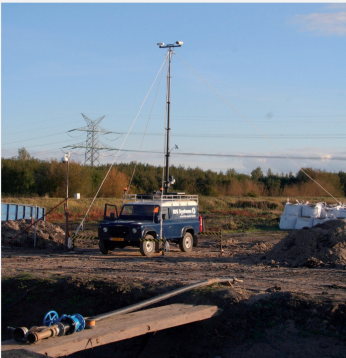
Figure 2-5: IDS system stabilized installation pylon (Stichting IJkdijk, 2010)
