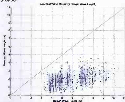
Figure 1: nowcast significant wave height vs. Design wave height per Area according to GWS
