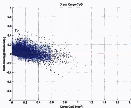
Figure 6:  $\delta_{\text{nowcast\_Measured}}$  vs. Measured x acceleration in Cargo CoG
