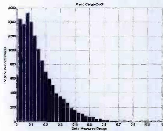
Figure 4: X acceleration in Cargo CoG occurrences vs.  $\delta_{\text{Measured\_Design}}$
