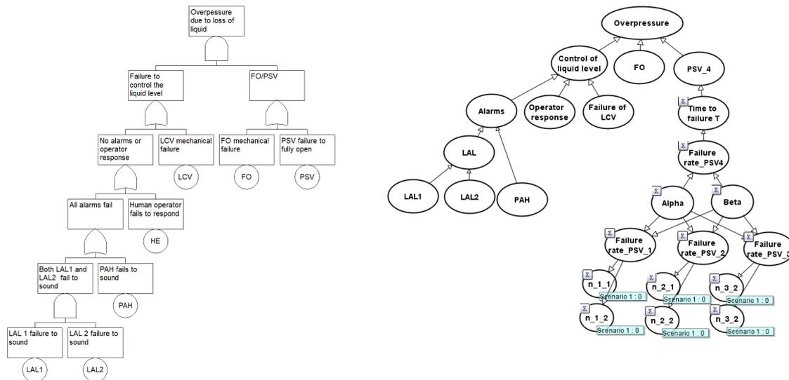
Figure 2a: The fault tree for the overpressure in the expansion vessel. Figure 2b: The BN extended by including hierarchical Bayesian analysis
