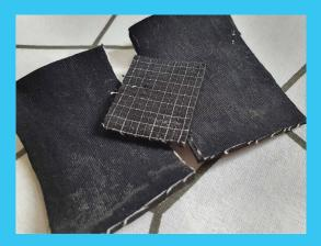
Photo of first neoprene prototypes using Vliesofix
