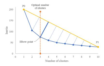
Figure 3.3 Optimal number of clusters identified with elbow method and mathematical method
