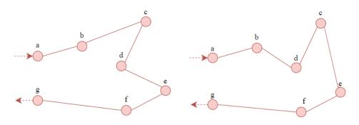
Figure 3.7 Schematic representation of a 2-opt swap move
