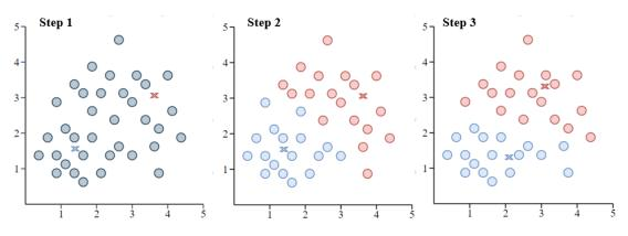
Figure 3.4 Schematic representation of each stage of the K-means clustering process
