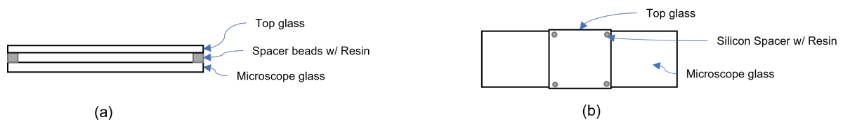
Figure A.2: (a) The side view of the cell (b) The top view of the cell
