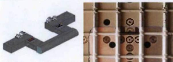
Figure 4 – Corrugation sensor alone (left) and as installed on the right rigid block (right)
