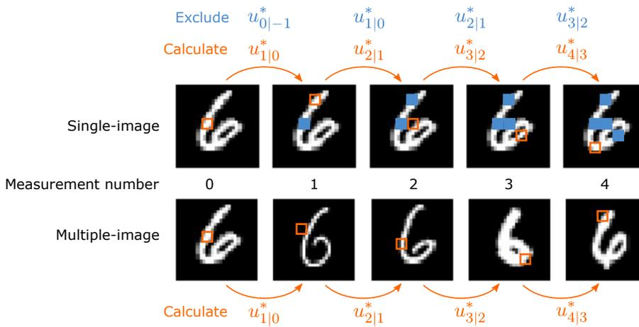
**Fig. 2.** Illustration of CLAMD in automated visual inspection using a single image (top) and multiple images from the same class (bottom), taken from the MNIST handwritten digit dataset [10]. After each measurement, the optimal next  $4 \times 4$ -pixel inspection region  $u_{k+1|k}^*$  is calculated. In the single-image case, previously inspected area is excluded, whereas the multiple-image case can have equivalent inspection regions for different measurement numbers.
