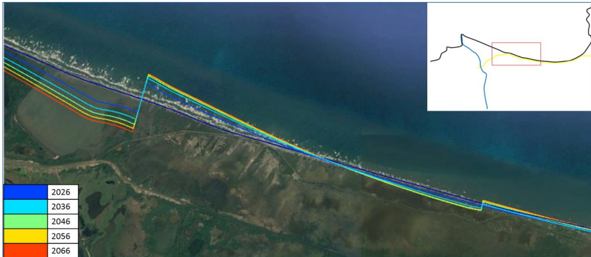
Figure 56: Coastline development over time with the alternative "Breakwater" at the critical locations
