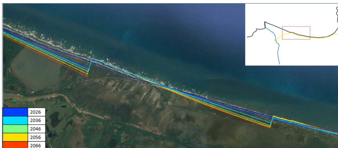
Figure 59: Coastline development over time with the alternative "Groin Field" at the critical locations
