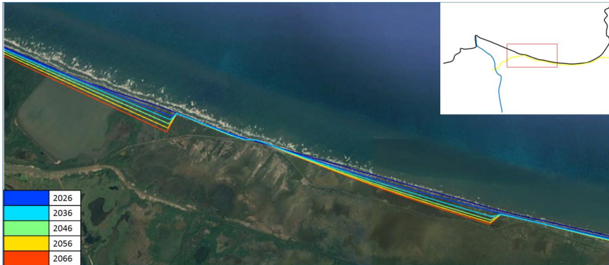
Figure 52: Coastline development over time with the alternative "Revetment" at the critical locations
