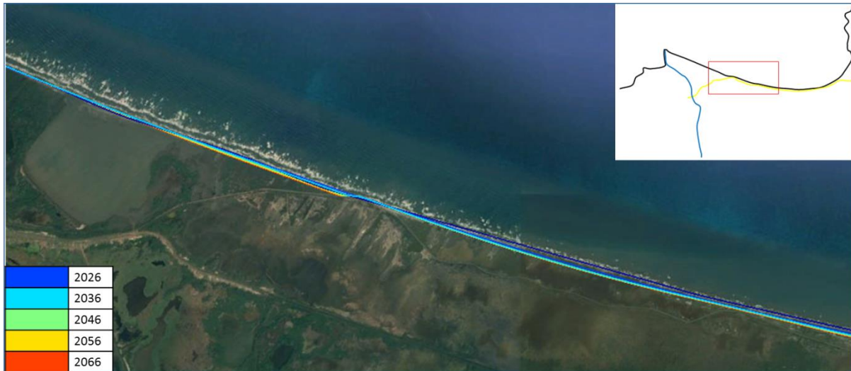
Figure 62: Coastline development over time for the alternative "Nourishment" at the critical locations
