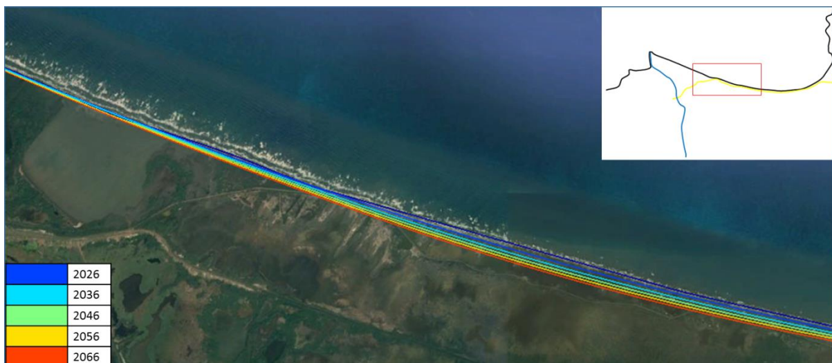
Figure 65: Coastline development over time with the alternative "Relocate Road" at the critical locations
