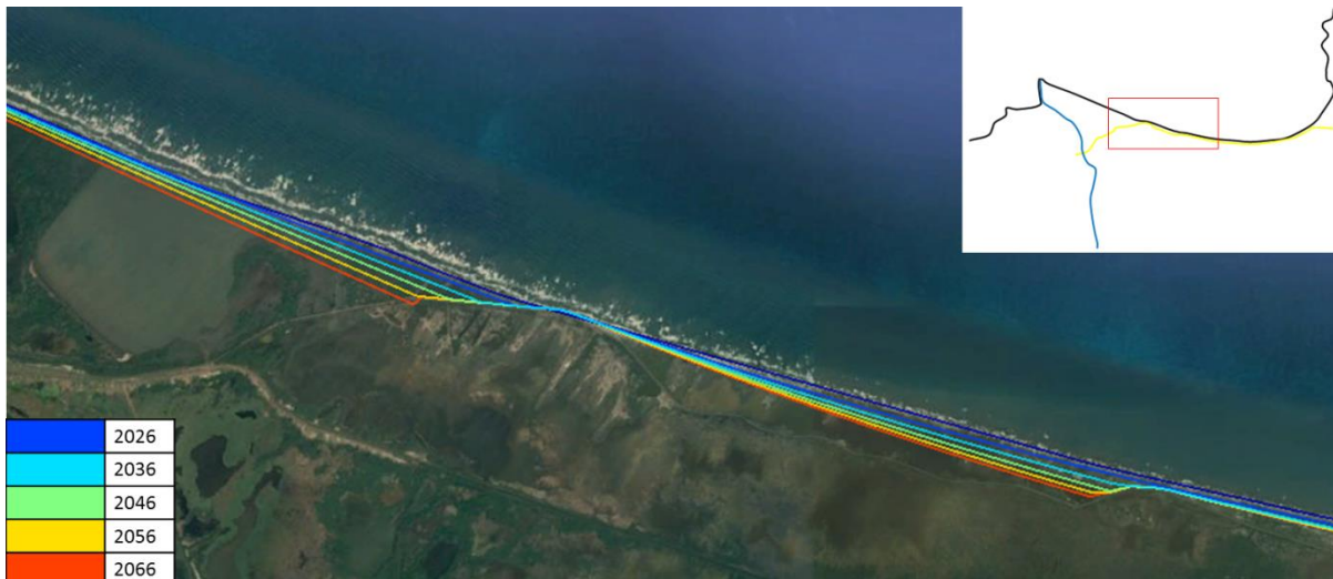
Figure 49: Coastline development over time with the alternative "Extension" at the critical locations
