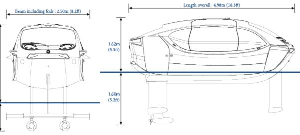
Figure 2: Dimensions of the seaBubble for seven passengers (SeaBubbles, n.d., b)
