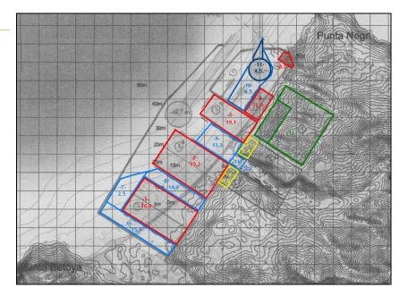
This results in a total volume of 69\*10<sup>6</sup> m<sup>3</sup> 'dredging' of land required, which is around 93% of volume of material required for reclamation (which remains the same at 74\*10<sup>6</sup> m<sup>3</sup>. The remaining percentages (soil material required for land reclamation) can be acquired by the necessity to level the surrounding terrain in an assumed slope of around 1:3.
