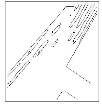
Container port entrance run Wave direction: 0°N Wave height: H<sub>2</sub>=2.25 m Contour lines: 0.5, 1 m
