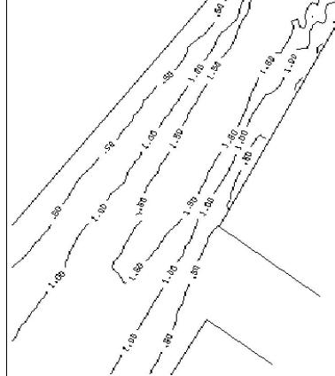
Improved container port entrance run Wave direction: 30°N Wave height: H<sub>s</sub>=2.75 m Contour lines: 0.5 - 2 m
