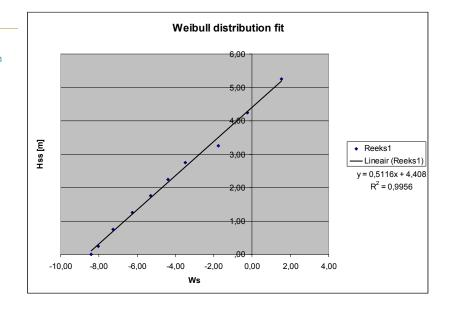
With the previously determined probability of failure p=0.1 in combination with the 1/475 year storm, the design storm wave height can be calculated on which the breakwater design will be based. This follows from:
