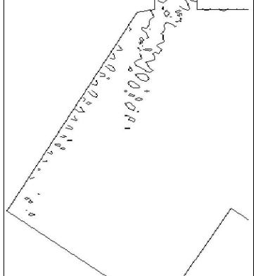
Improved bulk port run Wave direction: 30°N Wave height: H<sub>s</sub>=2.25 m Contour lines: 1.5 m
