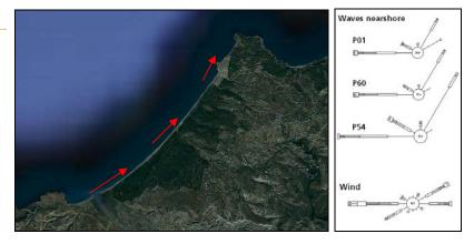
This particular breakwater orientation already limits the possibilities for the approach channel alignment as determined earlier: option 4, where the approach channel was oriented around 75°N is with this decision almost not feasible.
