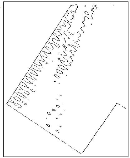
Bulk port run Wave direction: 30°N Wave height: H<sub>c</sub>=2.75 m Contour lines: 1.5, 2 m
