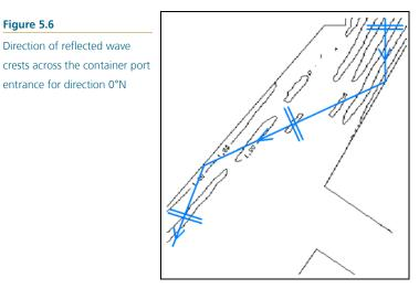
Reflection will be an important aspect to take into account when reviewing the wave conditions at the entrance. There is considerable variation in isolines, which indicates standing waves across the container port entrance. At locations close to the breakwaters, wave heights higher than the incident wave heights occur due to (almost complete) reflection. The direction of the (reflected) wave propagation in-port is clearly visible in the simulation runs.
