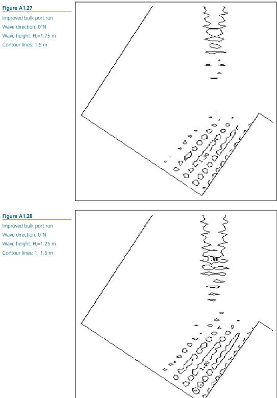
Improved bulk port run Wave direction: 0°N Wave height: H<sub>s</sub>=1.25 m Contour lines: 1, 1.5 m
