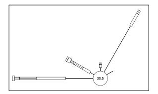
From the above it is evident that there are two main resulting wave directions: NNE and W-WNW. However, the waves from NNE have a smaller significant wave height and peak period than the waves arriving at the project location from W-WNW. This will be taken into consideration when designing the different port items.
