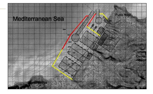
Regarding the exact composition of the rubble mound breakwaters (e.g. the use of armour units), a decision will be made in the next chapter, in combination with the technical design. The above outlined indications of the breakwater types are at this stage sufficient to make an in-port wave study possible.
