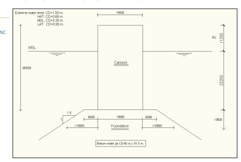
The length of the caisson can be chosen somewhat arbitrarily. However, several sources (under which Goda) recommend caissons lengths up to 45 - 50 m. at maximum. To limit the number of caissons that needs to be sunken down, this latter caisson length of 50 m. will be used within the design.
