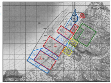
This already results in an increase in 'dredging' to 88\*10<sup>6</sup> m<sup>3</sup>, which is 119% of the reclamation. However, there would be large height differences present between the container terminal height at the inland basin (13, 14) around CD +3 m. and the surrounding terrain, up to CD +55 m. This would make the construction practically difficult.
