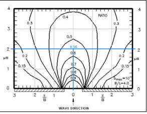
From the figure above it is clear that with this approach the diffraction coefficient  $K_d$  is around 0.56. However, this is a (too) low value. Due to reflection and the limited space behind the breakwater this value should actually be higher. At this point, the current visual approximation method from the Coastal Engineering Manual falls short: it lacks proper ground to assess the far from standard container port entrance layout.
