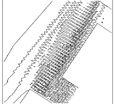
Improved container port entrance: berths run Wave direction: 30°N Wave height: H<sub>s</sub>=1.25 m Contour lines: 0.5 – 1 m
