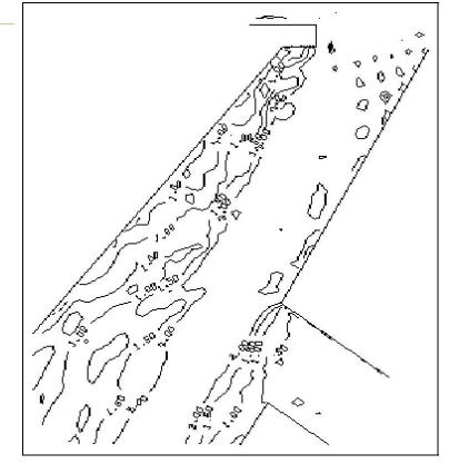
Container port entrance run Wave direction: 330°N Wave height: H<sub>c</sub>=1.25 m Contour lines: 0.5, 1 m
