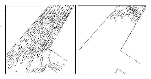
Incident waves with a height of H=2.25 m. also do not pose problems for (all of) the berths. At the entrance itself it is clear that there inevitably is wave action present, and a particular pattern develops. The standing wave pattern could lead to hindrance to entering vessels. However wave dampening measures reduce this as much as possible, and in the lee of the breakwaters tugs can fasten to the vessels up to wave heights of H $\leq$ 2.75 m.
