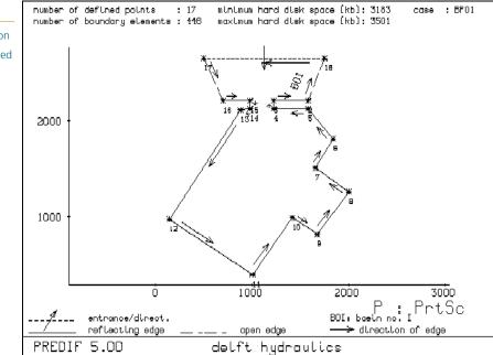
In the schematization, several specific rules had to be taken into account. The breakwater width needs to be at least  $0.5*L_{\rm max}$  to avoid ill-posed equations [DIFFRAC-2DH MANUAL].
