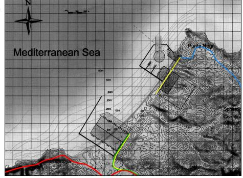
It is emphasized that the container berths required dredging until a depth of CD -17,4 m. Special attention has to be paid that also the northern container terminal berths reach the appropriate depth. This part has been hatched in the figure above.
