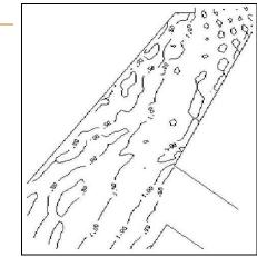
This scenario will be of special importance later on when assessing berths (3) and (4) deeper in-port (see figure 5.7). When reviewing the container port entrance, it appears that incident waves from  $30^{\circ}$ N with wave heights larger than H=1.75 m. will lead to a scenario where the wave height in the lee of the breakwaters is too high for tugs to tie up (H>2.0 m.).
