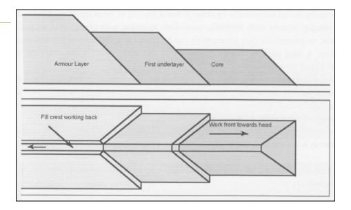
For this layer, controlled placement of stones with a weight of W=3-6 t. will have to be executed. For the lower cross-sectional profile of the breakwater, use can be made of sidestone-dumping vessels. The upper profile of the breakwater will again be constructed from the landside onwards, by using dump trucks and excavators for controlled placement.
