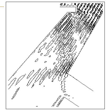
Container port entrance run Wave direction: 300°N Wave height: H<sub>c</sub>=1.25 m Contour lines: 0.5 - 1 m
