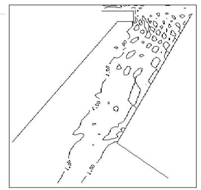
Container port entrance run Wave direction: 30°N Wave height: H=1.75 m Contour lines: 0.5 - 2 m
