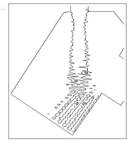
Container port entrance run Wave direction: 0°N Wave height: H=1.25 m Contour lines: 0.5, 1 m
