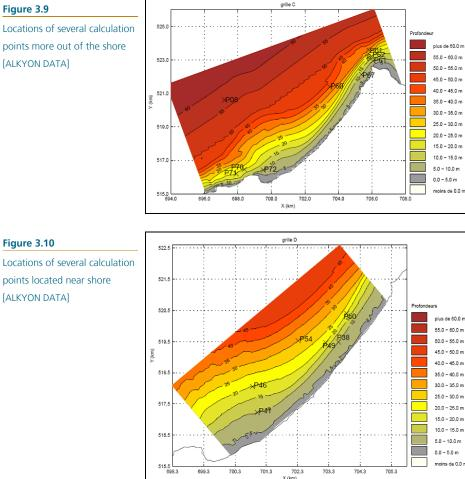
For all the available different output locations, the significant wave height  $H_s$  [m] and the spectral peak period T<sub>p</sub> [s] are presented in annex 2.1. Here, for the port design three relevant locations along the coast have been selected in order to describe/quantify the main wave climate and it's parameters at more or less the same depth along the coast. These are:
