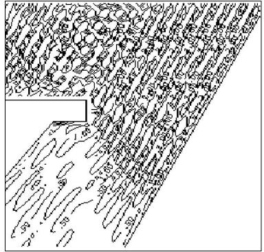
Improved container port entrance run Wave direction: 330°N Wave height: H<sub>s</sub>=2.25 m Contour lines: 0.5 – 1.5 m
