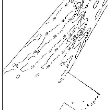
Improved container port entrance run Wave direction: 330°N Wave height: H<sub>s</sub>=1.25 m Contour lines: 0.5 - 1 m
