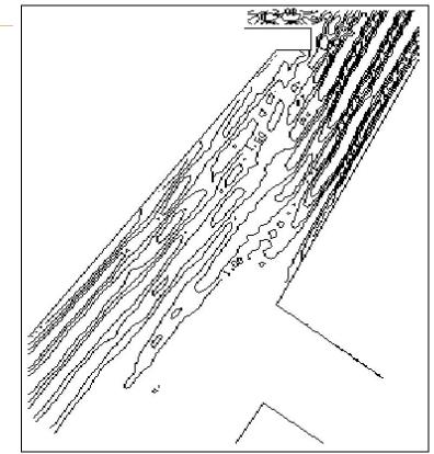
Container port entrance run Wave direction: 30°N Wave height: H\_=1.25 m Contour lines: 0.5 - 1.5 m
