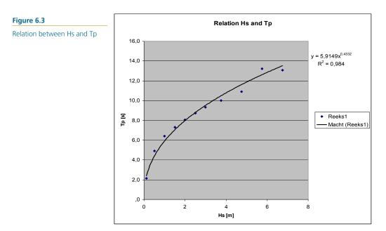
With the relation  $y=5.9149^*x^{(0,4332)}$  from the figure above and the design storm wave height of  $H_{s_{51/475}} = 8.45$  m. the accompanying wave period can be calculated as follows:
