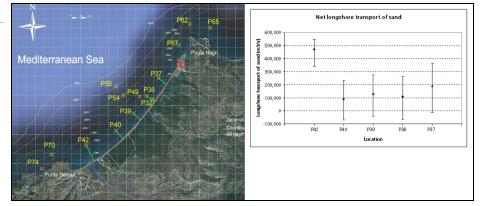
It is assumed that the Rio Kert should always be able to discharge into the Mediterranean Sea because of its large catchment area and thus discharge and sediment load. This could be realised for example with the help of an outlet stabilisation. It is deduced from this that the location around the Rio Kert outflow is not suitable for the construction of the new port.
