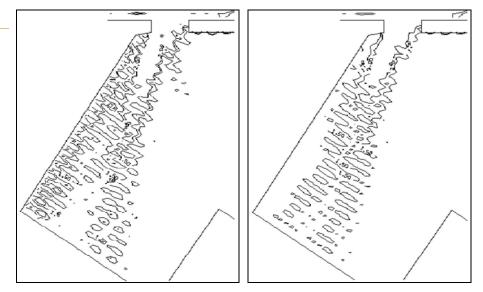
When assessing the influence of the wave dampening measures from the direction of 0°N, also some (small) improvements are directly visible, see the figure below.
