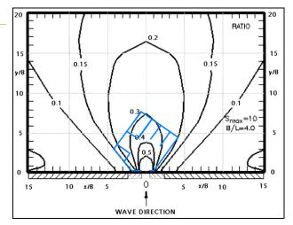
It should be noted that in these diffraction diagrams from [USACE, 2002], reflection of (diffracted) waves has not yet been taken into account. Besides this, the diffraction diagrams are valid for breakwaters with unrestricted space in the lee side behind the gap. This is not exactly the case in the bulk port layout. Also, the diagrams apply for an orientation of the two breakwater tips at 180°.
