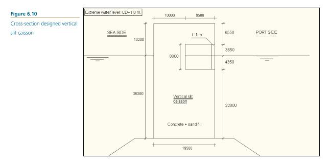
As a last remark, some earlier made assumptions need to be checked. It was calculated before that the stability of the caisson was achieved even for the most severe conditions (H=8.45 m.), the ULS.
