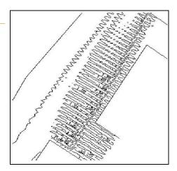
Waves from directions other than 30°N do not penetrate far enough in-port to arrive at berths (3) and (4). So the only downtime for these berths is caused by waves from 30°N larger than H=0.75 m. This specific scenario occurs for only 7.74% of time (see wave data table P60 in annex 2) and results in an availability for these specific berth of 92.26%.
