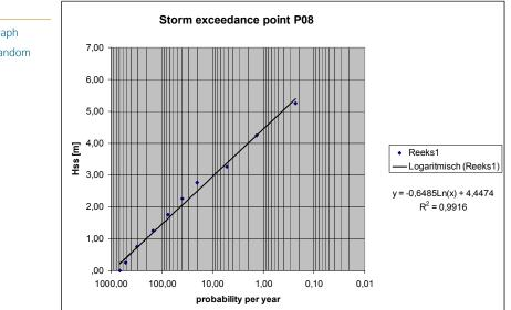
Subsequently, this analysis can be improved by using the Weibull distribution [VERHAGEN *et al.*, 2009]. This distribution has been proven to be the most robust. This has been done accordingly, and the results are presented in figure 6.2. This figure has been constructed by using the last column of table A2.13.
