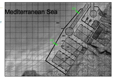
The two cross-sections are chosen at the most critical locations: where the water depth is the largest, and for C2 also the wave action on the inside of the breakwater due to wave reflection.
