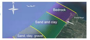
In zones I (purple), bedrock is present. This the case at Punta Negri and Punta Betoya. Especially the bedrock at Punta Negri (andesite) is very hard and difficult to dredge (see white arrow). Close to the coastline, this rock is present at depths less than CD -20 m.
