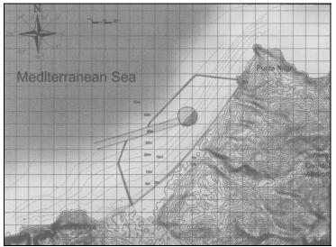
Still the preferred approach channel layout is number 1, where the stopping length can be acquired by using the space inside of the breakwaters for the oil terminal. So at first glance, this direction will be more or less maintained as preferable approach channel alignment, when taking into account the layout of the breakwaters, hydrodynamic forces and morphological aspects. It is emphasized that the exact angle is still subject to variation in the design later on.
