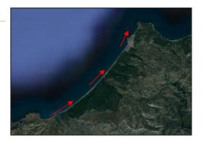
However, the instantaneous sediment transport depends on the environmental conditions occurring at that time: for example, waves from 0-30°N lead to an instantaneous longshore sediment transport in the opposite direction (to the southwest).
