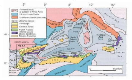
About 25 km. to the west of the project location, a major tectonic fault is present: the Nekor Fault. At the project location itself, a smaller fault is present, the Taliwine. This is between the location of Punta Betoya to the southwest and the mouth of the Rio Kert. The exact location offshore and the activity are unknown [ALKYON DATA]. It is assumed that this fault runs from north to south, extending the line northwards in the figure below.
