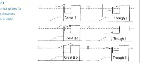
The extended Goda-formulas can be used in combination with several modification factors  $\lambda$ depending on the structural type. These factors also differ for various stages and scenarios where the e.g. the wave crest or trough hits the structure. The table below presents these factors for the different stages.
