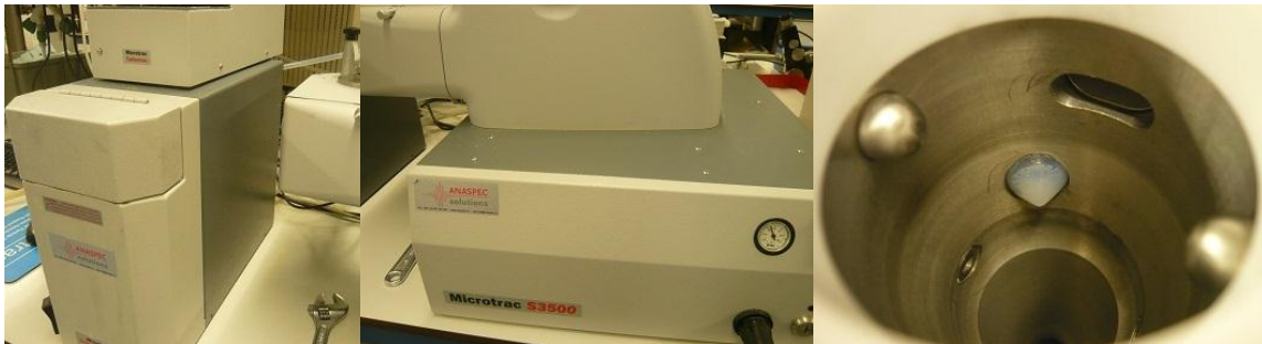
Figure 5-5: Photo showing SDC (left), Microtrac S3500 PSA (middle) and deliver point (right)
