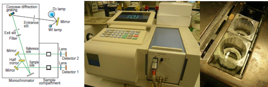
Figure 5-15: U-2900 spectrophotometry schematic (left), overview (middle) and sample cuvette (right)
