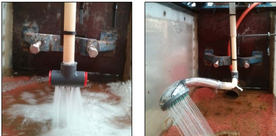
Figure 5.34 – Special nozzle designs in an unsubmerged situation
