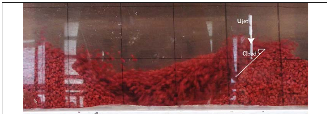
Figure 6.8 – Observed penetration profile for p_j = 0.023 bar and v_{trail} = 0.07 m/s (Test 1)
