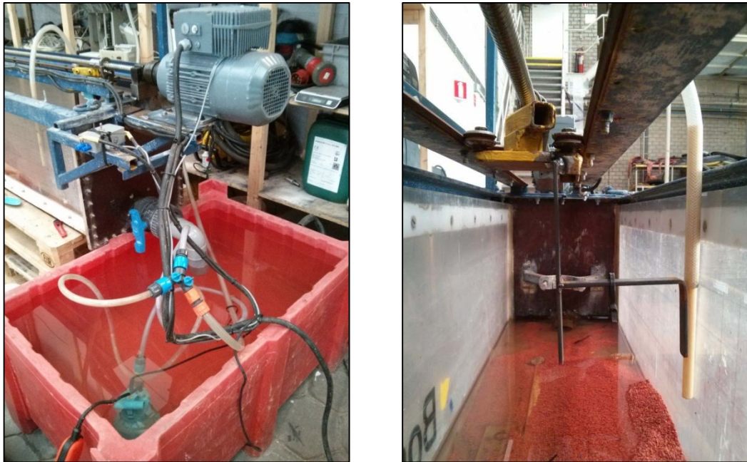
Figure 3.5 – Pumping system (left) and cart with jet nozzle (right, empty tank)
