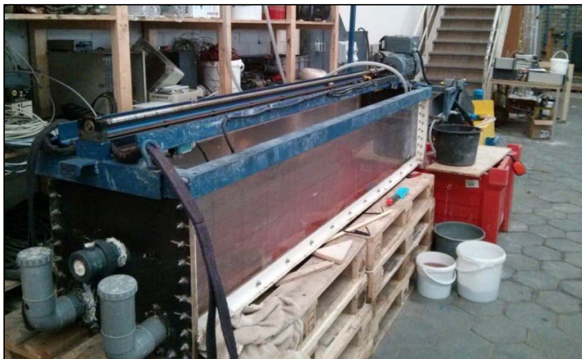
Figure 3.4 – Water tank used for small scale tests
