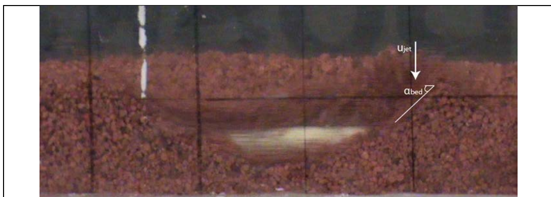
Figure E.2 – Observed penetration profile for p_j = 0.008 bar and v_{trail} = 0.05 m/s
