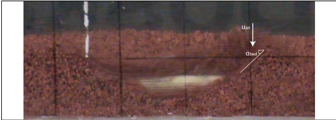
Figure 6.9 – Observed penetration profile for p_j = 0.008 bar and v_{trail} = 0.05 m/s (Test 2)
