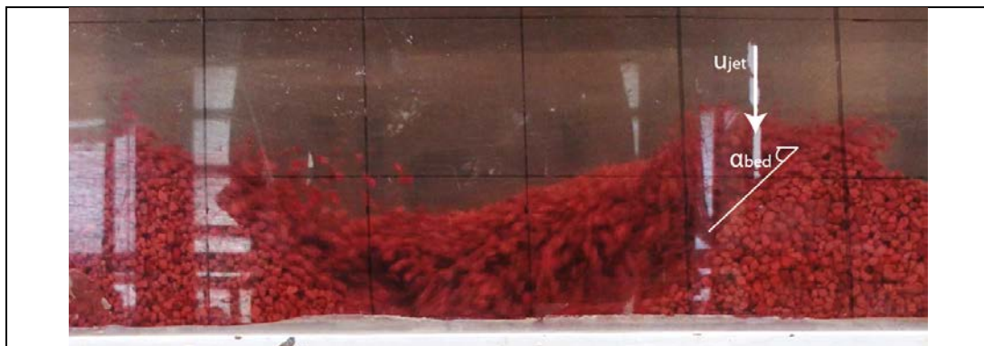
Figure E.1 – Observed penetration profile for p_j = 0.023 bar and v_{trail} = 0.07 m/s
