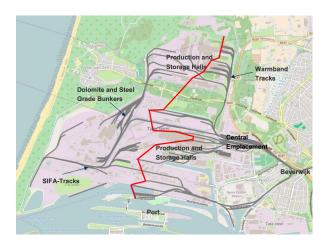
Figure 1.2: Rail network at Tata Steel IJmuiden. The red line indicates the non-physical separation between the network West (left) and the Central (right).
