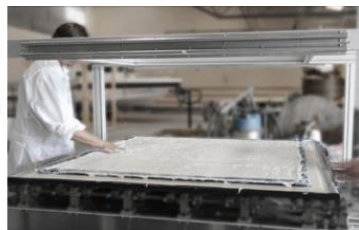
From digital model to physical concrete panel ( http://adapa.dk/ )
