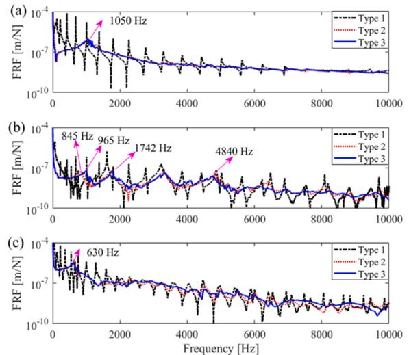
**Fig. 12.** FRFs with rail constraints type 1, 2 and 3 at accelerometer 1 in the (a) vertical, (b) longitudinal and (c) lateral directions. The pink arrow in (a) shows the vertical resonance mode at 1050 Hz, the arrows in (b) indicate the longitudinal resonance modes at 845 Hz for type 2 and 965 Hz for type 3, and the arrow in (c) shows the lateral resonance mode at 630 Hz.
