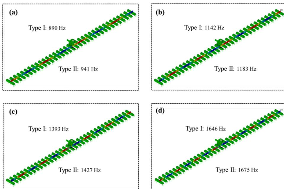
**Fig. 17.** Rail longitudinal compression modes with rail constraint models type I and II. (a) 890 Hz for type I and 941 Hz for type II with the same mode shape; (b) 1142 Hz for type I and 1183 Hz for type II; (c) 1393 Hz for type I and 1427 Hz for type II; (d) 1646 Hz for type I and 1675 Hz for type II.
