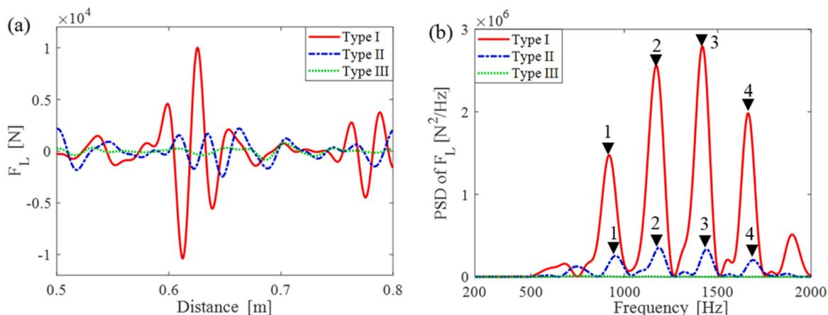
**Fig.16.** Longitudinal wheel-rail contact forces with rail constraint models type I, II, III in the spatial and frequency domains. (a) Spatial domain; The fluctuation amplitude of longitudinal contact force with type III is significantly smaller than those with type I and II. (b) frequency domain. The marks (▼) indicate the characteristic frequencies of the contact forces with type I and type II.
