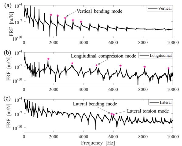
**Fig. 10.** FRFs with the rail constraint type 1 at accelerometer 1 in the (a) vertical, (b) longitudinal and (c) lateral directions. In this figure, (★) show some examples of vertical bending modes, longitudinal compression modes, lateral bending and torsion modes.
