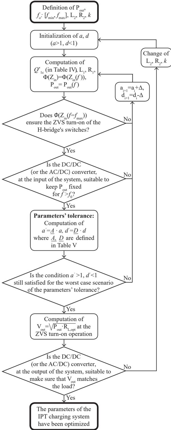
Fig. 6. Flow chart that summarizes the selection process of the optimized parameters for IPT charging systems based on the coefficient  $a$ , or  $d$ .
