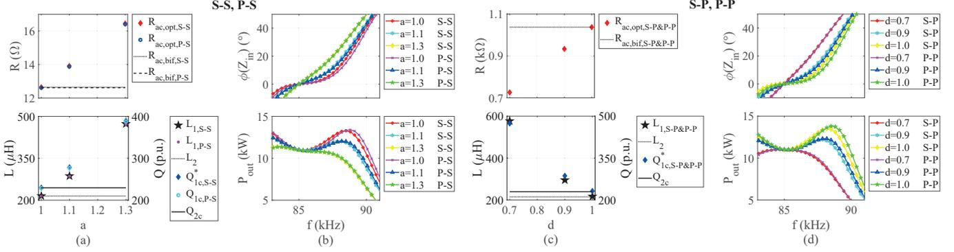
Fig. 2. 11 kW wireless battery charging systems at different values of either the coefficient  $a$  for the S-secondary in (a),(b), or  $d$  for the P-secondary in (c),(d). (a),(c): optimum load, coils' inductance and quality factor. (b),(d): phase angle of the input impedance and output power depending on the frequency.
