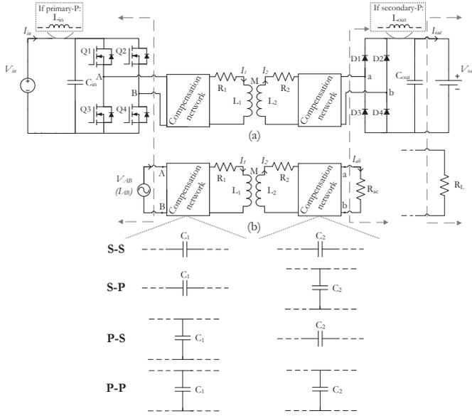
Fig. 1. Equivalent circuit of the four basic compensation networks (S-S, S-P, P-S, P-P): (a) complete system, (b) phasor equivalent circuit.
