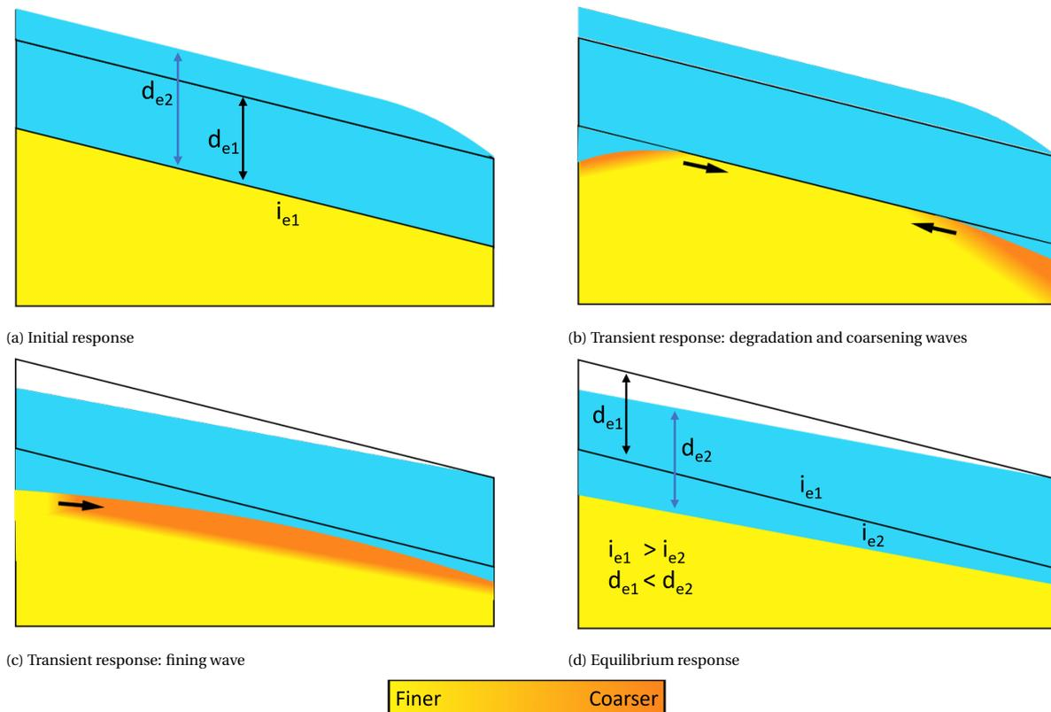
Figure 6.3: The initial, transient and equilibrium response of a river with bi-modal sediment to S1: an increasing discharge.
