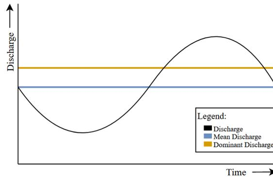
Figure 3.1: A simple hydrograph with its mean and dominant discharge.
