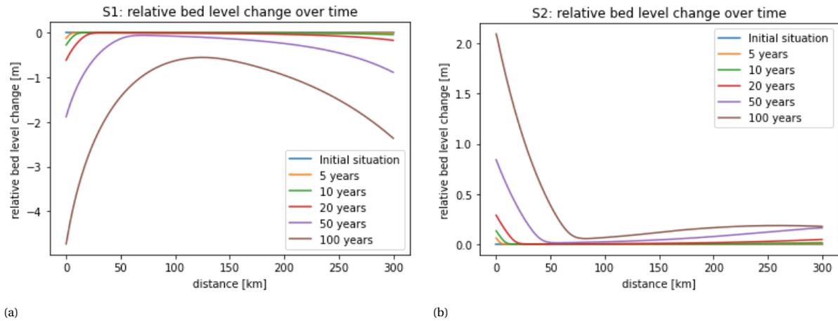
Figure 5.1: Relative development of the river channel bed over a period of 100 years for an increasing discharge (a) and a decreasing discharge (b).
