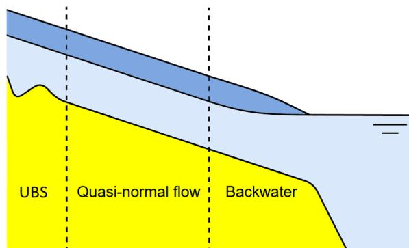
Figure 3.3: The upstream boundary segment, quasi-normal flow segment and backwater segment in a river reach with a hydrograph during base flow (light blue) and peak flow (dark blue) (Blom et al., 2017).
