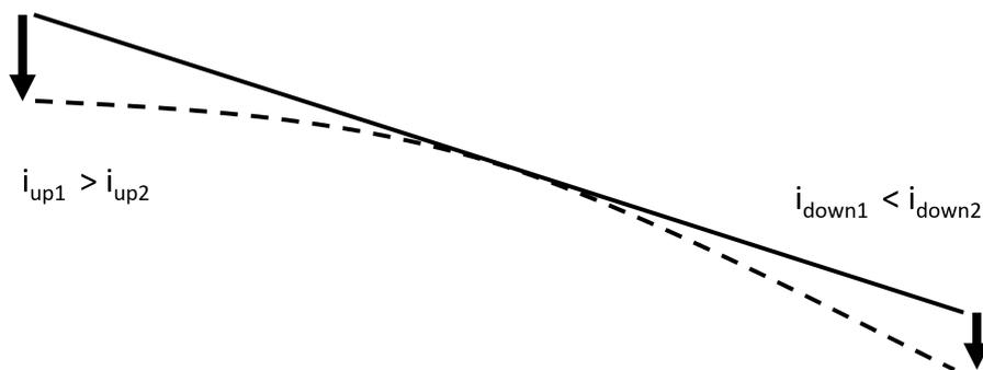
Figure 3.8: When a river degrades at both the up- and downstream end, this results in a decreased bed slope upstream and an increased bed slope downstream.
