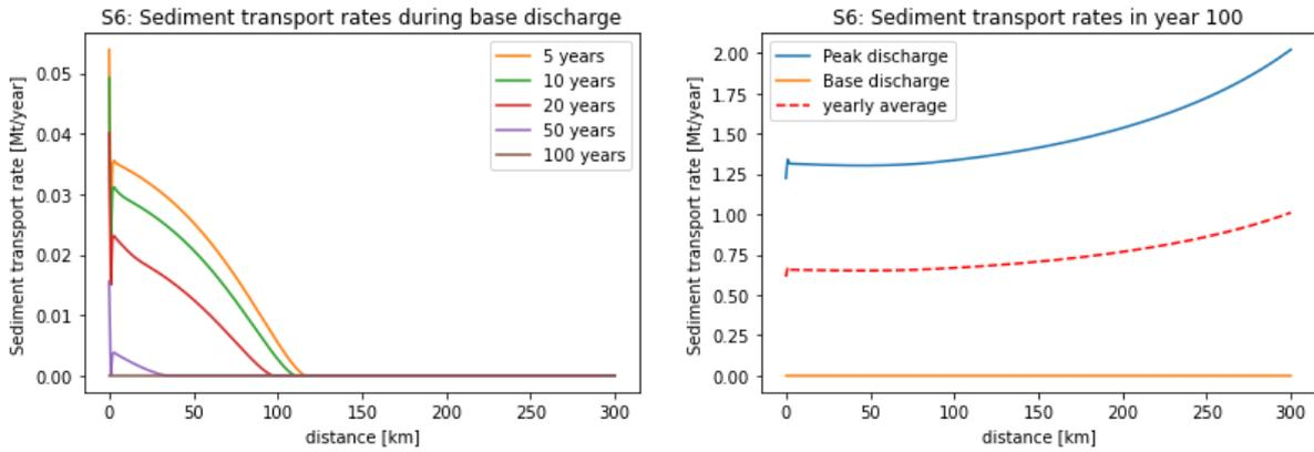
(a) Sediment transport rate during base discharge over the river reach at different moments in time.
