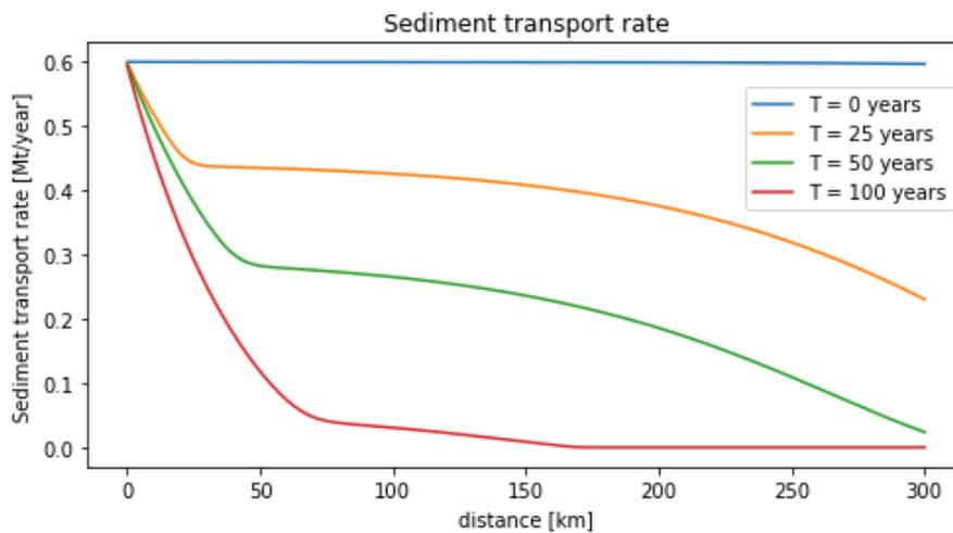
Figure 5.4: The sediment transport rate for multiple years over the river reach for scenario 2.
