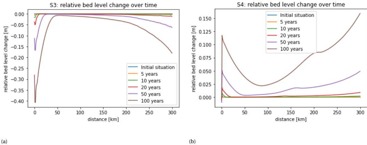
Figure 6.6: Relative bed level change compared to the initial situation for an increased variability (a) and a decreased variability (b) of discharge over a period of 100 years.
