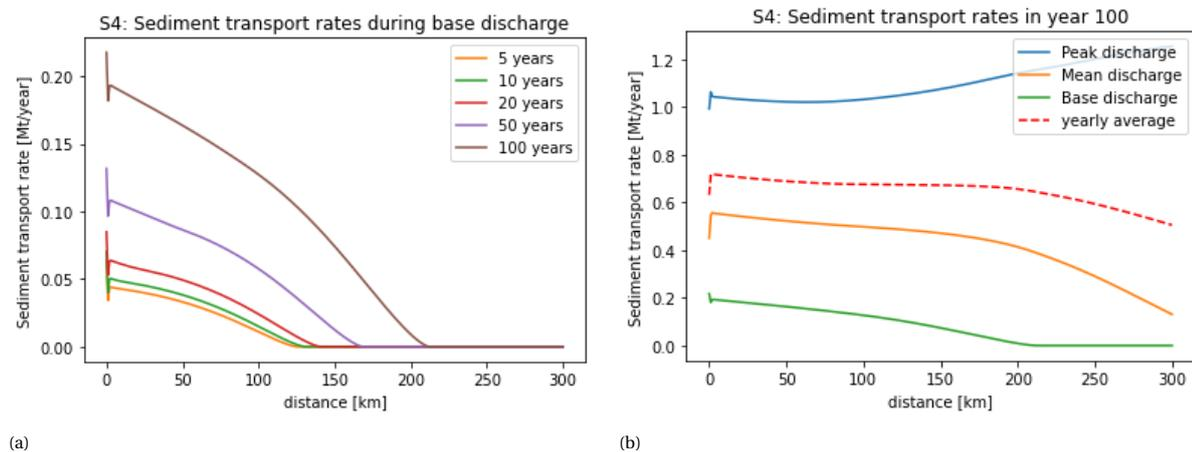
Figure 5.9: Sediment transport rates during base discharge at different moments in time (a) and sediment transport rates in the modelled year 100, including the yearly average (b) for S4: a decreasing water discharge variability.
