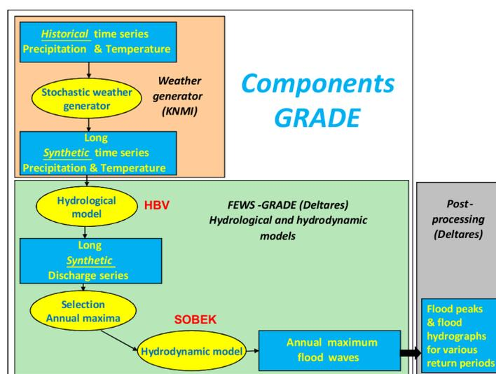
Figure 2.6: The components of GRADE (Hegnauer et al., 2014).
