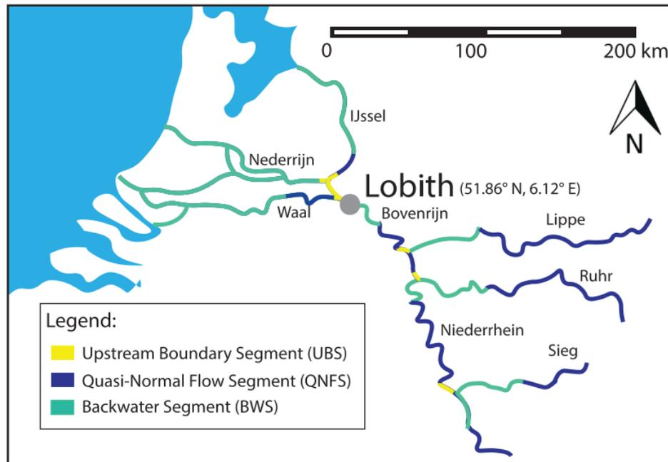
Figure 3.5: Schematic of the lower Rhine indicating the different flow segments (Arkesteijn et al., 2019).
