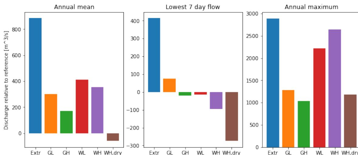
Figure 2.9: Change in discharge in 2085 compared to the reference period (1956-2006) for the annual mean (MQ, left), Lowest 7 day flow (NM7Q, middle) and annual maximum (MHQ, right).
