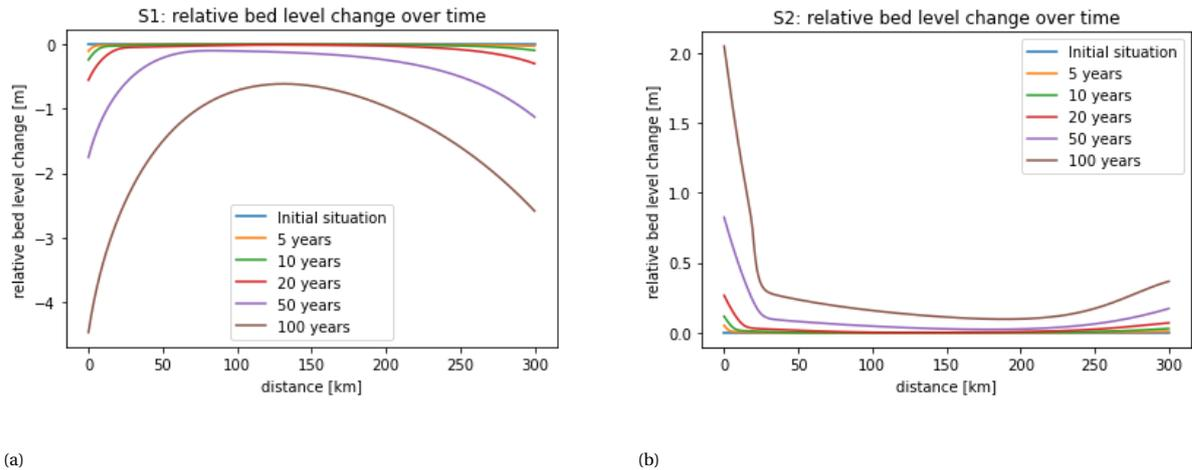
Figure 6.1: Relative development of the river channel bed over a period of 100 years for an increasing discharge (a) and a decreasing discharge (b).
