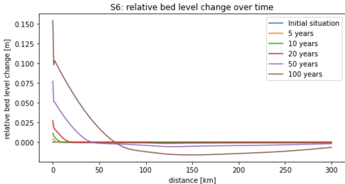
Figure 5.11: Relative bed level change compared to the initial situation for a decreased base discharge of  $500 \text{ m}^3/\text{s}$ .
