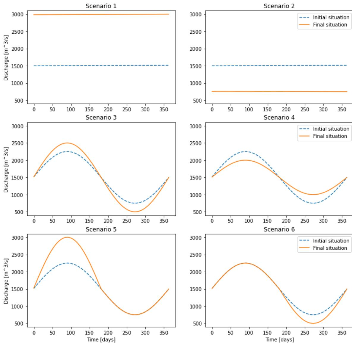
Figure 4.1: The initial hydrograph and the hydrograph after 100 years for the 6 scenarios.
