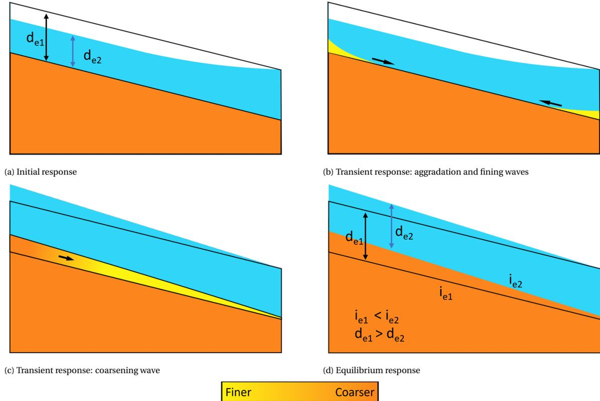
Figure 6.4: The initial, transient and equilibrium response of a river with bi-modal sediment to S2: a decreasing discharge.
