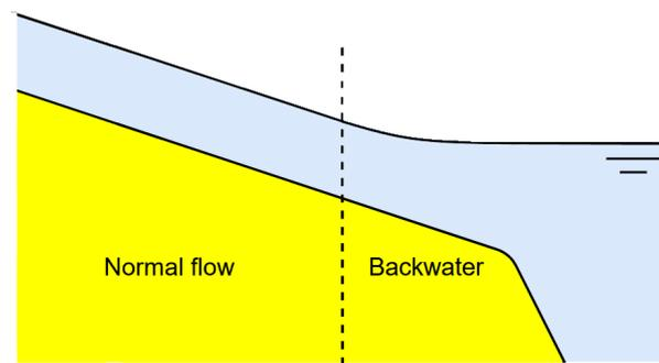
Figure 3.2: The normal flow segment and the backwater segment in a river with a single constant discharge. (Blom et al., 2017)
