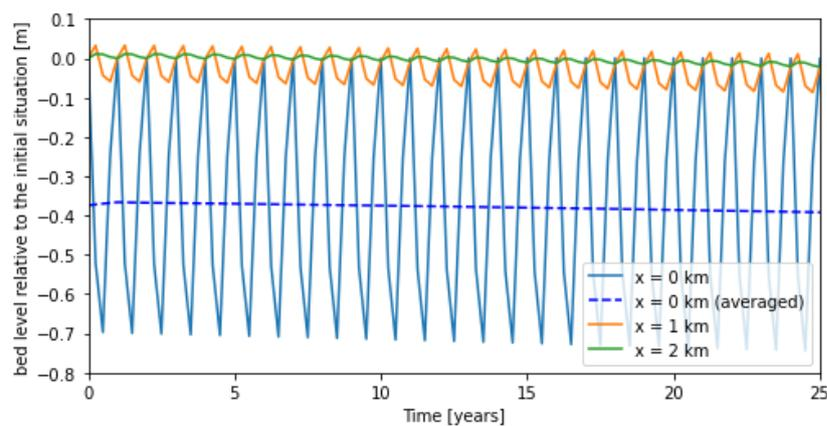
Figure 5.8: Relative bed level change over time for 3 locations at the upstream end of the river reach. The effect of the upstream boundary segment dampens out in downstream direction.
