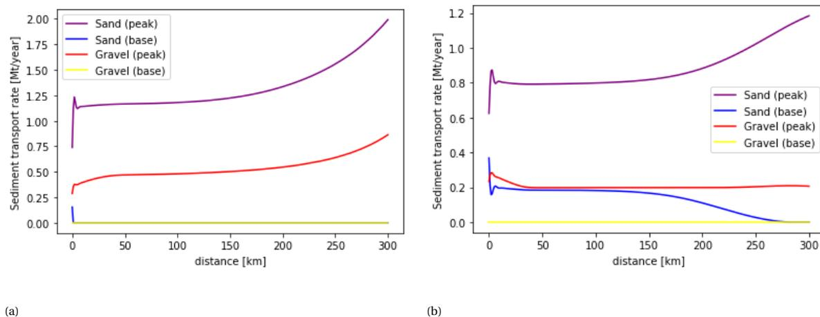
Figure 6.8: Sediment transport rates in the year 100 for S3: an increasing discharge variability (a) and S4: a decreasing discharge variability (b).
