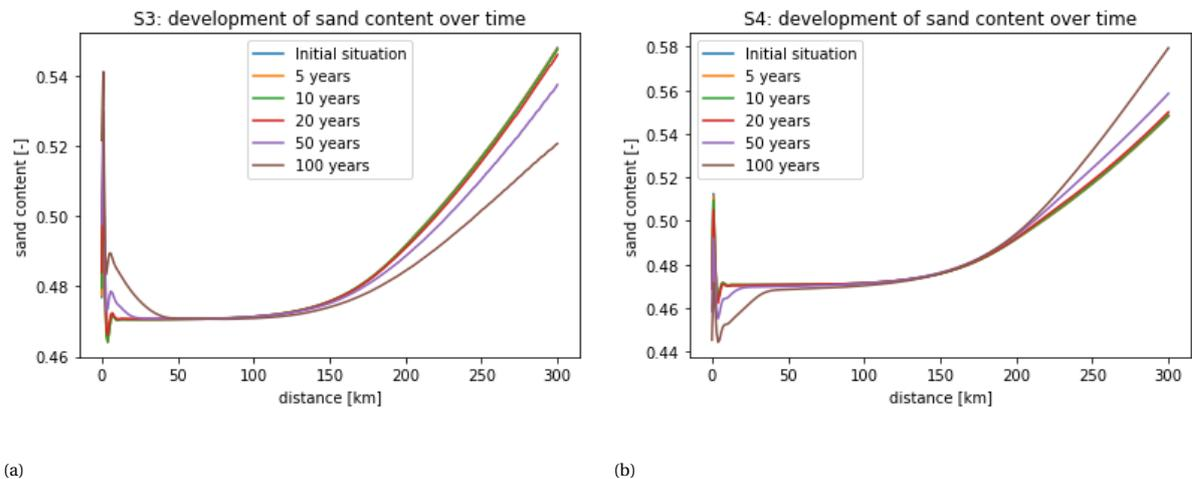
Figure 6.7: Sand content of the river bed for various moments in time. With (a) showing S3: an increasing discharge variability and (b) showing S4: a decreasing discharge variability.
