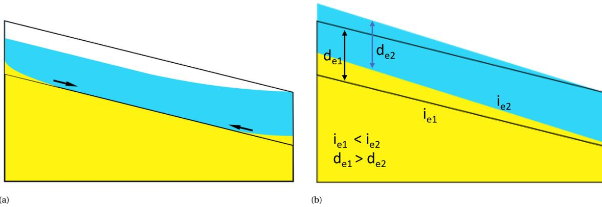
Figure 5.3: The transient (a) and equilibrium (b) response to a river reach with a fixed downstream water level and sediment supply due to a decrease of water discharge.
