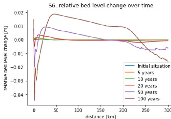
Figure 6.12: Relative bed level change compared to the initial situation for S6: a decreasing base discharge.
