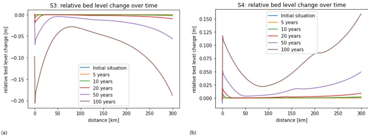
Figure 5.7: Relative bed level change compared to the initial situation for an increased variability (a) and a decreased variability (b) of discharge over a period of 100 years.
