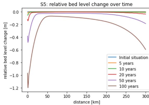
Figure 6.9: Relative bed level change compared to the initial situation for S5: an increasing peak discharge.
