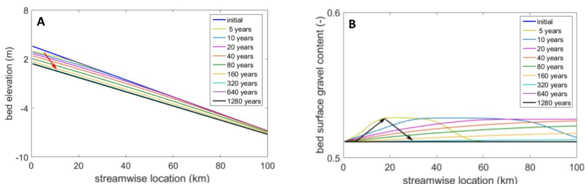
Figure 3.7: Bed elevation (A) and bed surface gravel content (B) response of a graded river to a 25% increase of the water discharge. Arrows show the direction of change in the transient phase (Siele et al., 2018)
