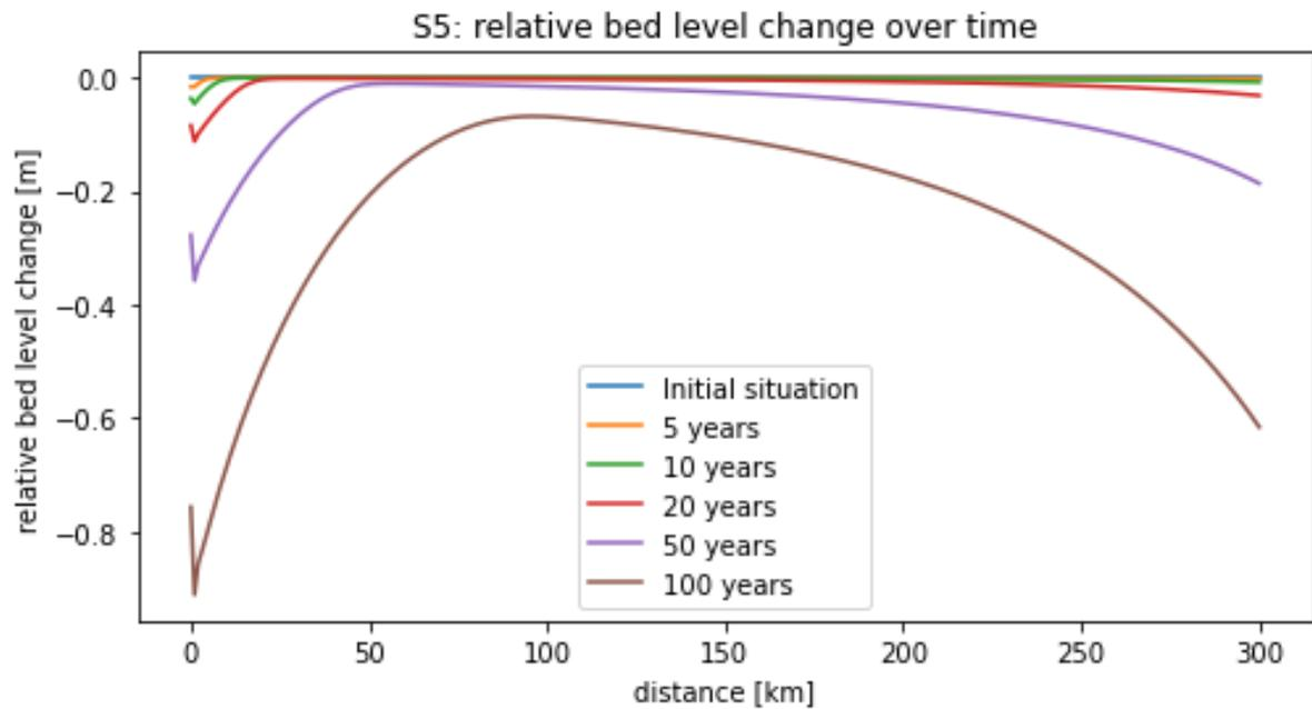
Figure 5.10: Relative bed level change compared to the initial situation for an increased peak discharge of  $3000 \text{ m}^3/\text{s}$ .
