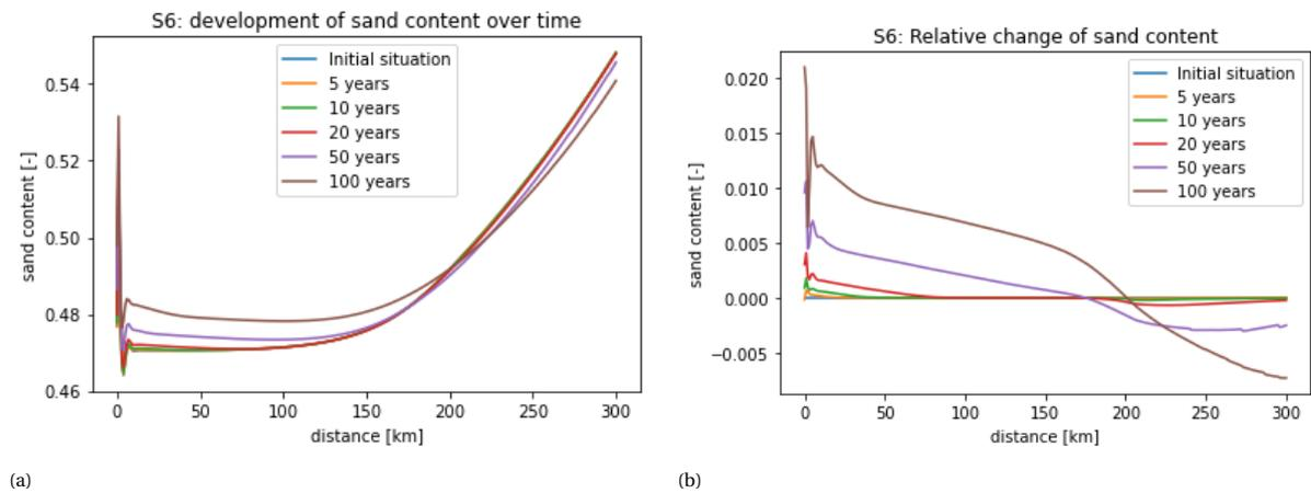
Figure 6.13: Sand content of the river bed for various moments in time for S6: a decreasing base discharge. With (a) the actual sand content and (b) relative to the initial sand content.
