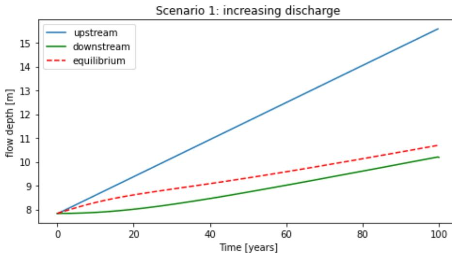
Figure 5.6: Development of the water level at the upstream end ( $x = 0$  km) and the downstream end ( $x = 300$  km) of the river reach for S1: an increasing constant discharge.
