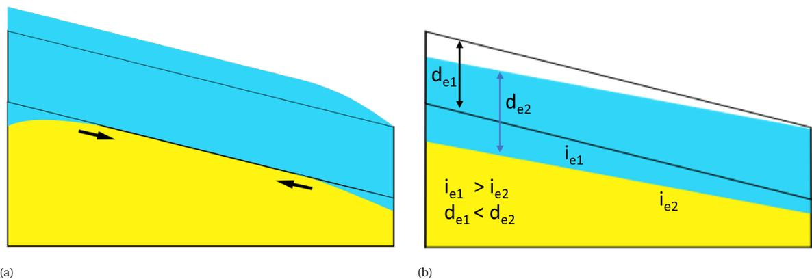
Figure 5.2: The transient (a) and equilibrium (b) response to a river reach with a fixed downstream water level and sediment supply due to an increase of water discharge.
