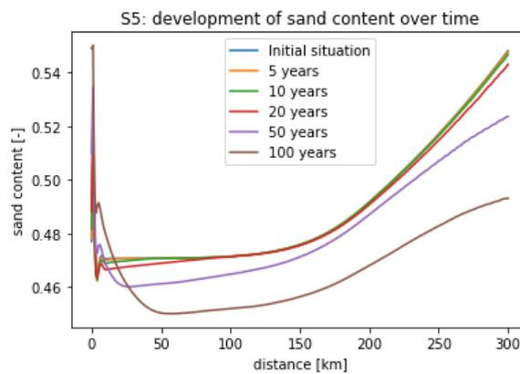
Figure 6.10: Sand content of the river bed for various moments in time for S5: an increasing peak discharge.
