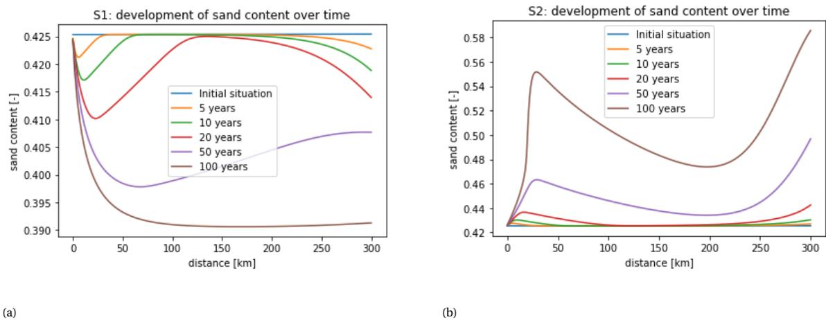
Figure 6.2: Sand content of the river bed for various moments in time. With (a) showing S1: an increasing discharge and (b) showing S2: a decreasing discharge.
