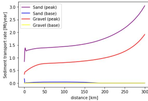
Figure 6.11: Sediment transport rates in the year 100 for S5: an increased peak discharge
