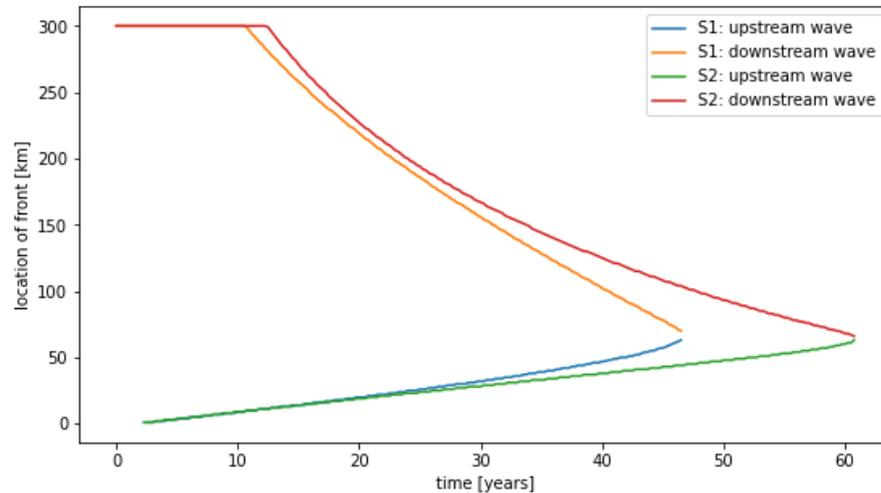
Figure 5.5: Location of the sediment wave front both up- and downstream for S1: an increasing discharge and S2: a decreasing discharge.
