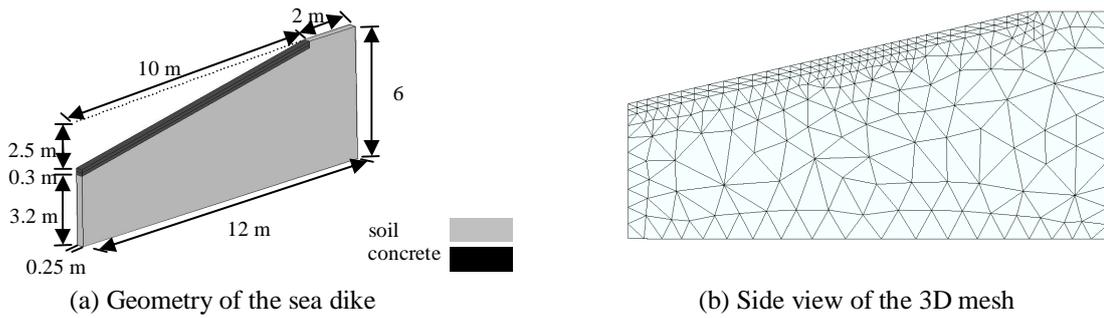
Fig. 2 Geometry of the sea dike and 3D mesh with plane strain boundary conditions
