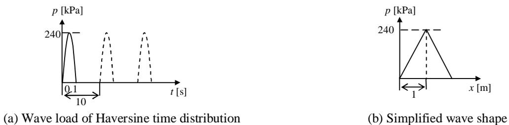
Fig. 1 Distribution of wave load
