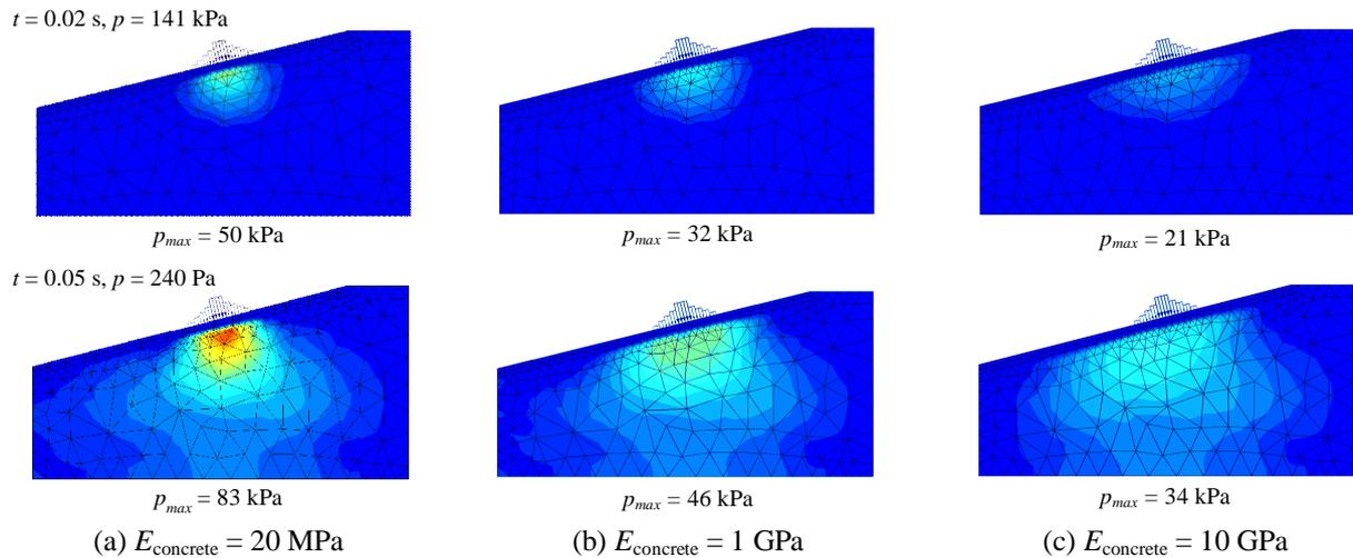
Fig. 4 Contours of excess pore pressure for different stiffnesses of concrete
