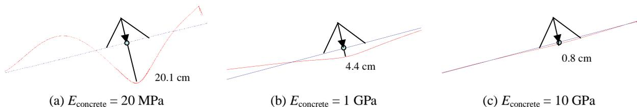
Fig. 3 Displacements at the surface of the concrete for the 10th loading cycle
