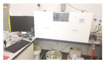
Figure E.1: MECO Cu plating equipment
