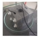
Figure 7.2: Leaking Si-air cell.
