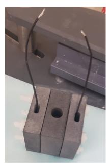
Figure 2.3: Isometric view of assembled Si-air cell
