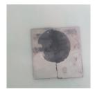
Figure 7.1: Broken Si sample.
