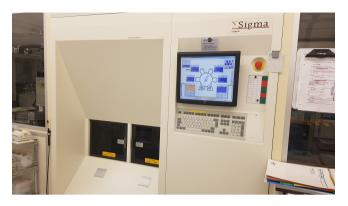
Figure E.4: Metal sputtering equipment in EKL lab
