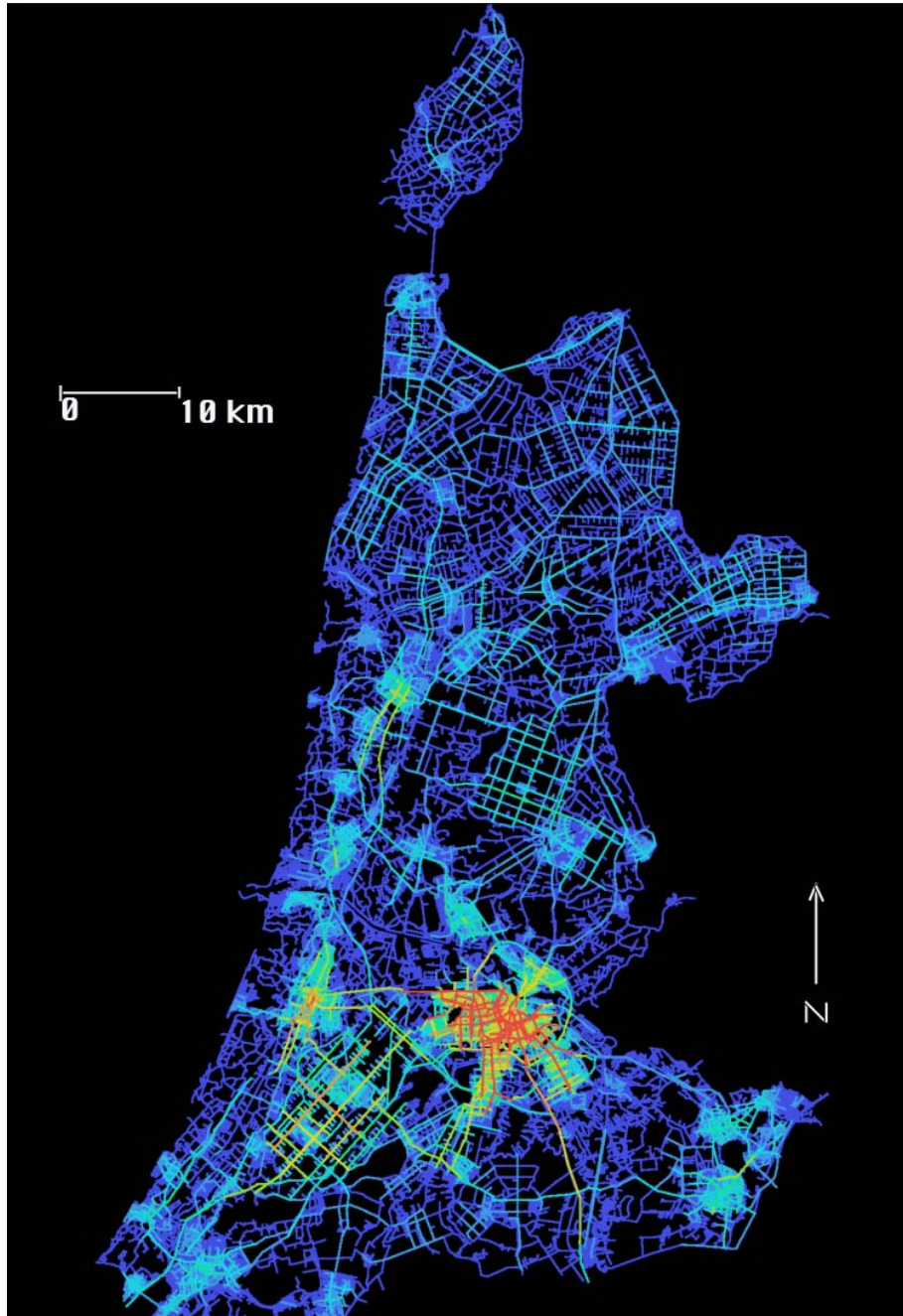
Figure 5: Local angular segment analysis with a topological radius 3 of the street and road network in the province of North Holland
