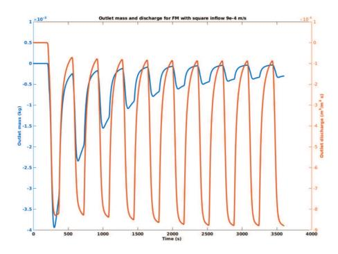
Figure 5: Outlet mass with outlet discharge rate obtained for FM
