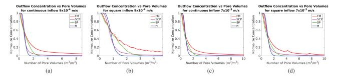
Figure 3: Measured outlet concentrations plotted against estimated number of flushed pore volumes for continuous and intermittent square wave inflow infiltration for different infiltration magnitudes.
