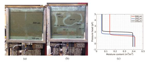
Figure 2: Laboratory scenarios for Homogeneous (a) and Heterogeneous (b) domains. Water retention curves optimized using DREAM<sub>ZS</sub> for sands of size  $100 \,\mu\text{m}$ ,  $250 \,\mu\text{m}$  and  $500 \,\mu\text{m}$  (c).
