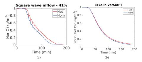
Figure 4: Normalized concentration against time duration for square wave intermittent infiltration in 41% of maximum pump flow rate on lab scale (a). VarSatFT validation for lab results (b).
