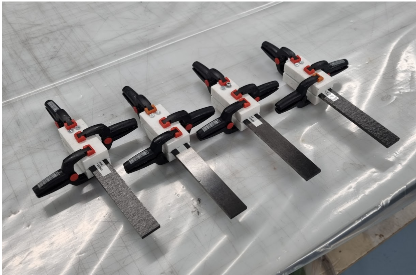
Figure 4.4: Using a Teflon mould for precise alignment, the aluminium tabs were bonded to the composite specimens.
