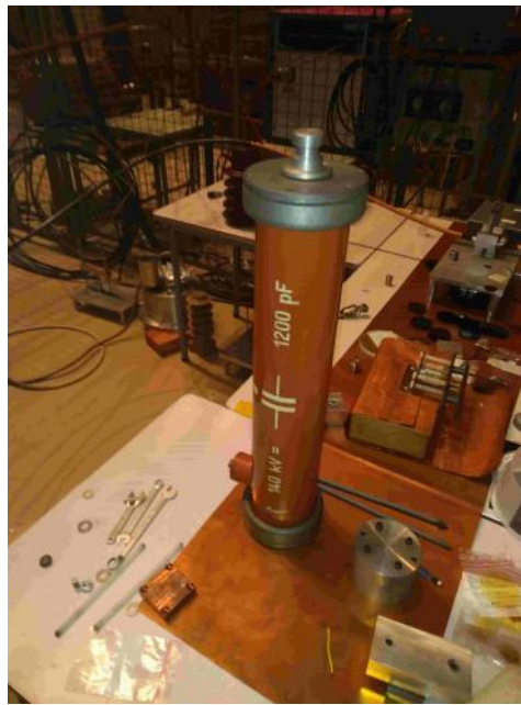
Figure 2.24: Termination capacitor of 1.2\ nF
