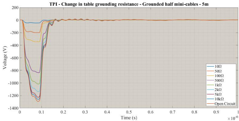
Figure 5.50: TPI - change in table grounding resistance - grounded half cables (PSCAD simulations)
