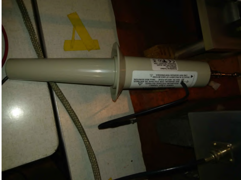
Figure 2.17: Tektronix P6015A high frequency high voltage probe - TU Delft
