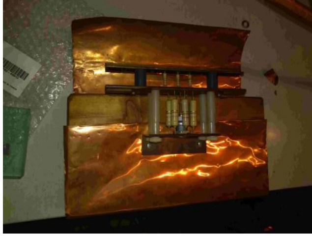
Figure 3.12: Pulse resistor R_p \approx 50 \Omega
