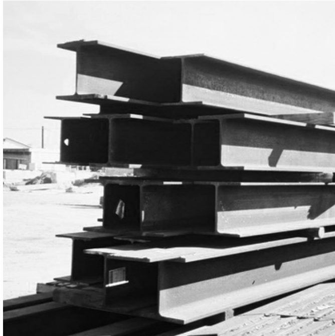
demountable, easily reusable steel beams
