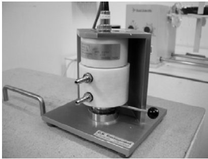
Figure 1 Rotronic station for RH measurement
