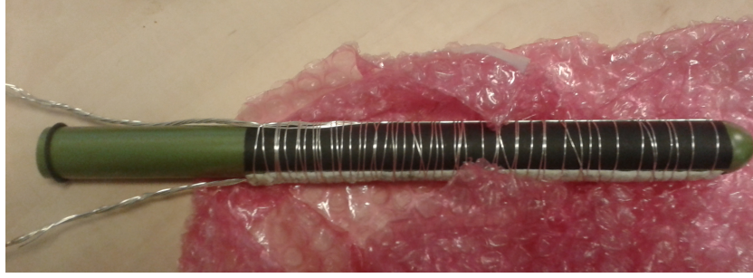
Figure 6.3: Picture of tubular SOFC
