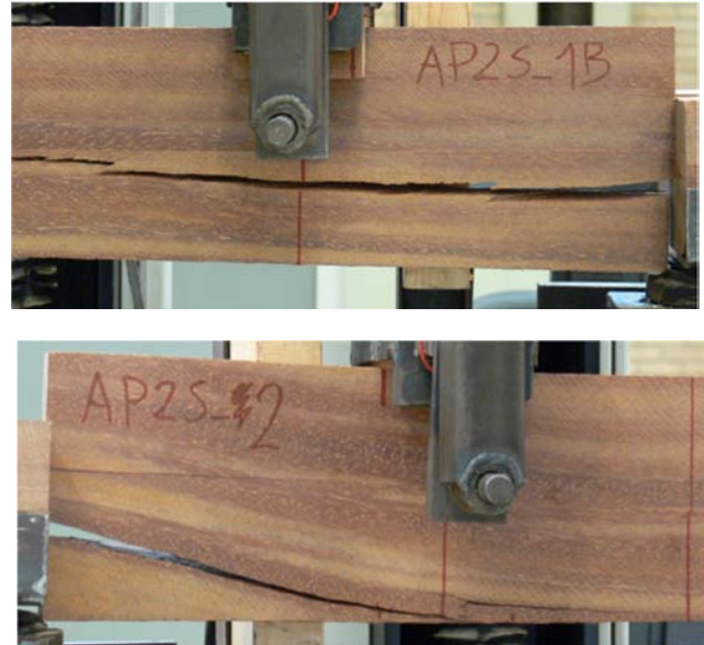
Figure 7a and b Tenon beams and crack patterns parallel to the grain and beam axis (a) and a different crack direction showing the influence of fibre angle (b).
