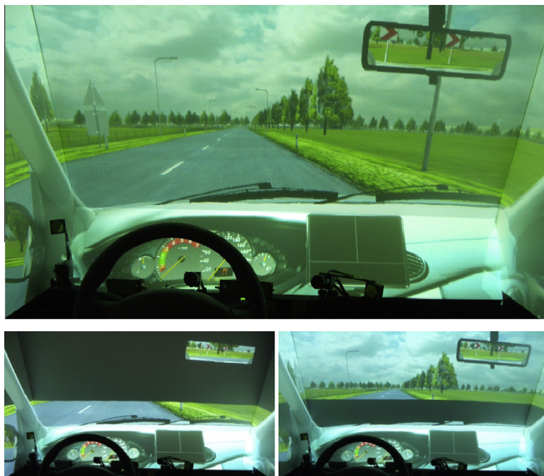
Fig. 1. Photos of the driving simulator; Top = control condition (C); Bottom left = near view (NV), all sight above 5 deg below the horizon was blanked; Bottom right = far view (FV), all sight under 4 deg below the horizon was blanked.
