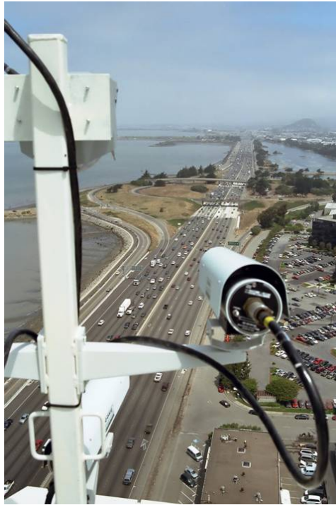
Figure 4.2: A digital video camera mounted on top of a building that overlooks I-80 is recording vehicle trajectory data.
