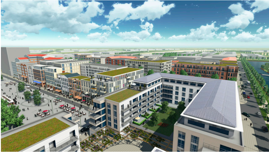
Figure 3.9: The BIM model of Leidsche Rijn Centrum. Because the model is so detailed, it can directly be used for visualization. (Image by Hfb [2016])
