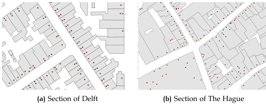
Figure 3.5: Differences between placement of point geometries between two municipalities.
