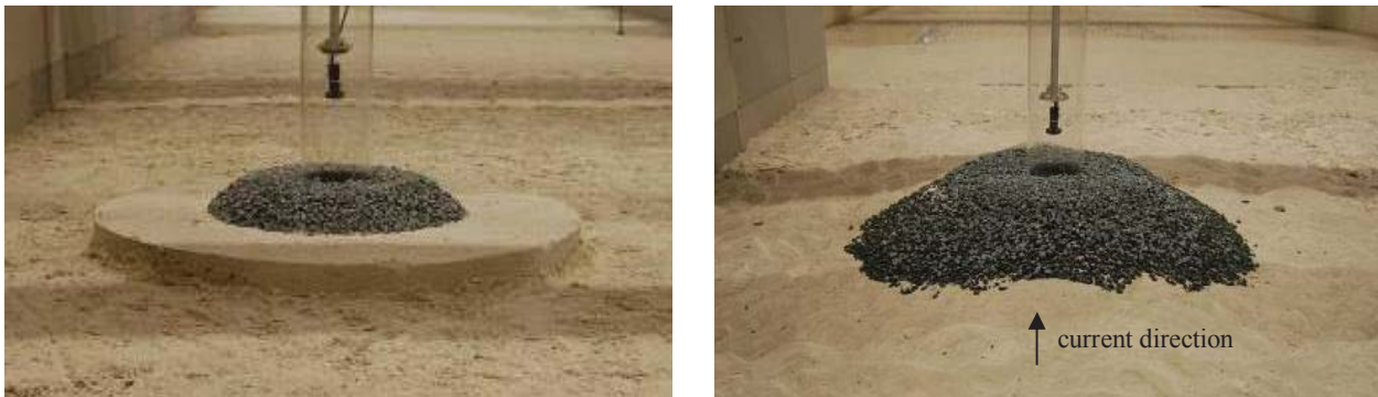
Figure 3: Photographs before (left) and after (right) test T-02 showing the redistribution of layout L03.
